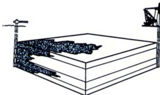
FIGURE 6.3 Oil can be recovered from reservoirs by pumping in steam, gas, or specialty chemicals. All methods face common problems posed by inhomogeneities in the rock containing the oil. Some major problems include poor vertical coverage, inefficient sweeping that bypasses pockets of oil, and severe channelling of fluids along fissures or highly permeable layers of rock. Chemical methods of compensating for these inhomogeneities would boost the yields and cut the operating costs of enhanced oil recovery. Courtesy, Amoco Production Company.
