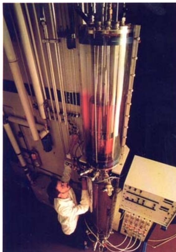
PLATE 4 Bioreactors that use mammalian cells, like this tower fermenter, are on the cutting edge of new biotechnology manufacturing processes. Courtesy, Cetus Corporation.
