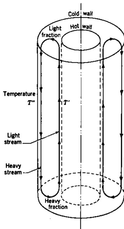
FIGURE C4 Schematic Diagram of Separation by Thermal Diffusion in a Clusius-Dickel Column.
