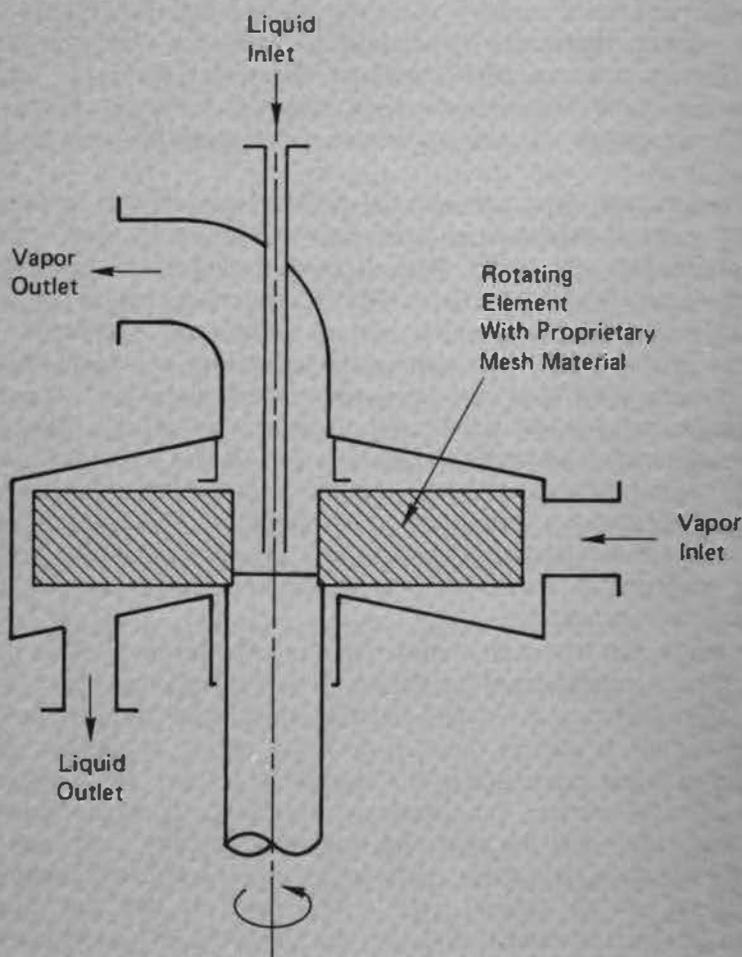
FIGURE S.5 Diagram of the ICI HiGee Column.
