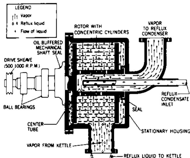
**FIGURE C.2** Centrifugal Multistep Solvent Extractor ("Podbielniak Contactor"). This diagram illustrates the principle of the Podbielniak Contactor for a vapor-liquid separation.
