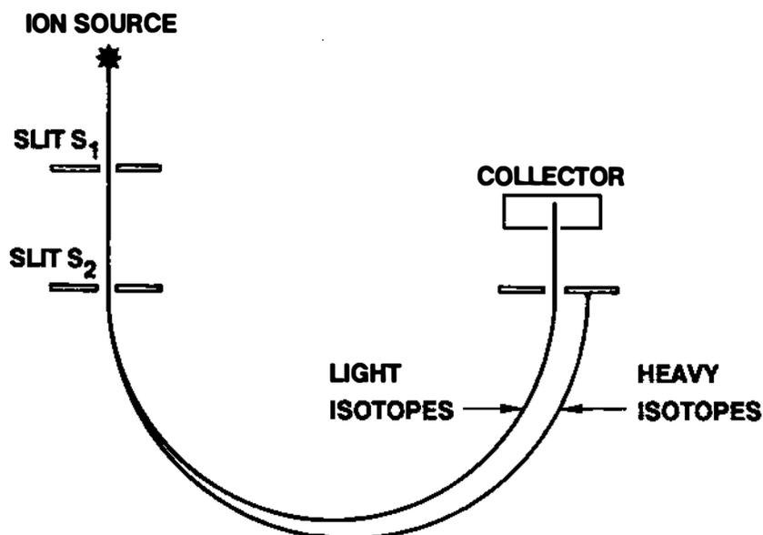
FIGURE C3 Mechanism of Electromagnetic Separation of Isotopes. When charged ions traverse a magnetic field (in the illustration the field is perpendicular to the page), their paths bend into circles whose radii are proportional to the mass of the ions.
