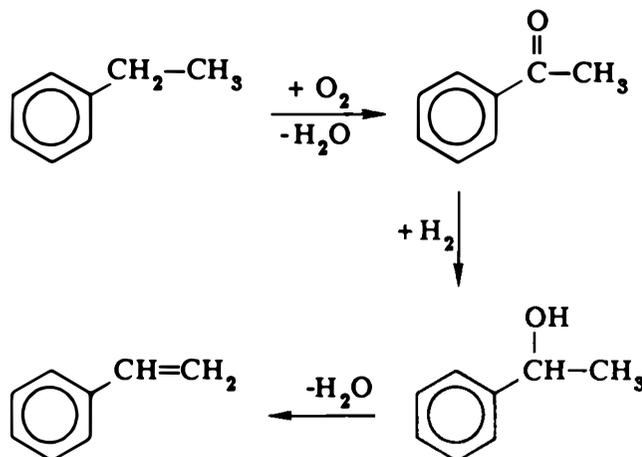
FIGURE C.1 Synthesis of Styrene from Ethylbenzene.
