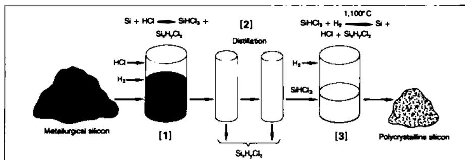
**FIGURE 4.3** Manufacture of Ultrapure Silicon: The production of polycrystalline silicon for the electronics industry involves several steps aimed at the reduction of impurities. These include [1] the reaction of metallurgical grade silicon to produce a mixture of chlorosilanes, [2] distillation of trichlorosilane, and [3] reduction of trichlorosilane to polycrystalline silicon.
