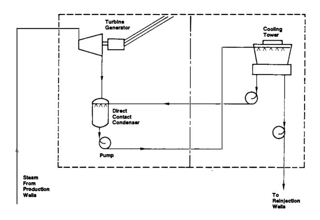
FIGURE C-1 Schematic Diagram of a Dry Steam System.
