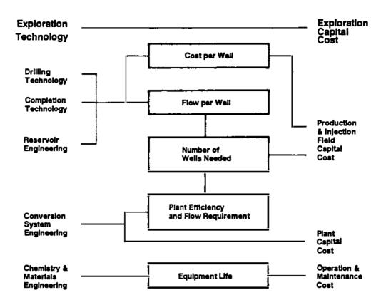
FIGURE 2-1 Geothermal Technology Cost Relationships.
