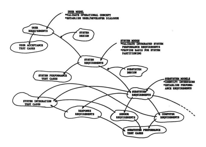
FIGURE 1 System acquisition life cycle for embedded systems.
