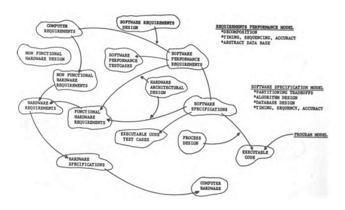
Figure 2 Software life cycle for embedded systems.
