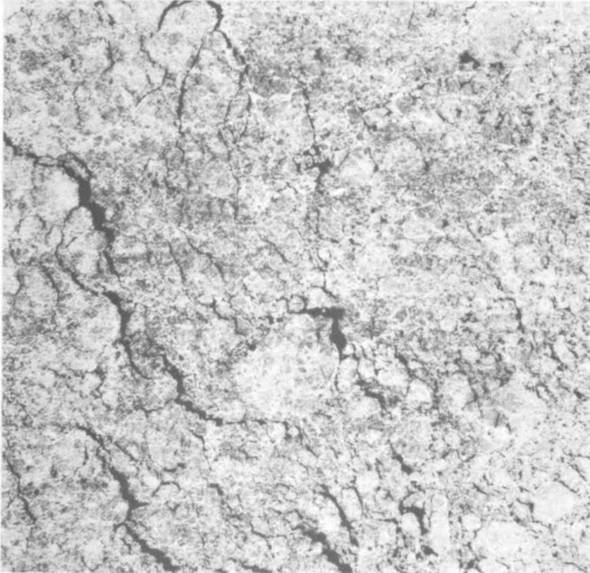
**FIGURE 6.2** A Seasat SAR image (Rev. 1382, October 1, 1978) of pack ice in the Beaufort Sea showing floes crossed by bright ridges and separated by dark leads. The very high return feature located just north of the center of the image is believed to be an ice island fragment in that known ice islands have been observed to give similar high returns. As ice islands are major hazards to offshore operations, it is very desirable to be able to track their movement.
