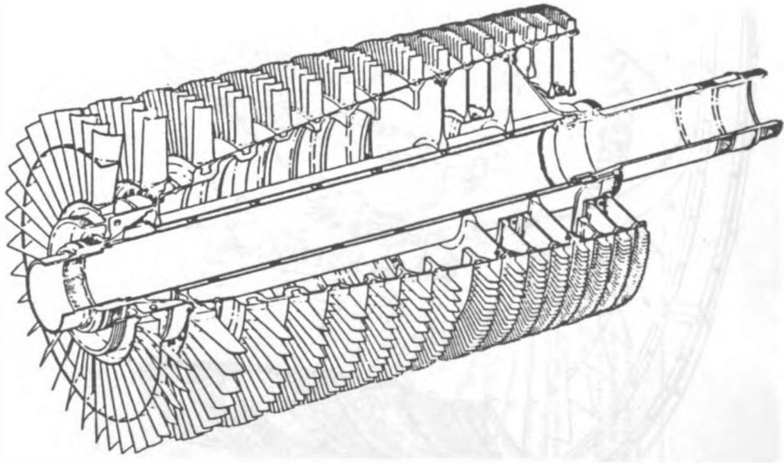
**FIGURE 17** Compressor rotor of a CF6-6 engine (courtesy of General Electric Company).
