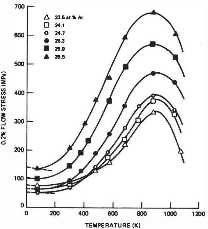
FIGURE 3 The effect of deviations from stoichiometry on the flow stress of Ni<sub>3</sub>Al and Ni<sub>3</sub>Ga at 77°K and room temperature (Noguchi et al. 1981).
