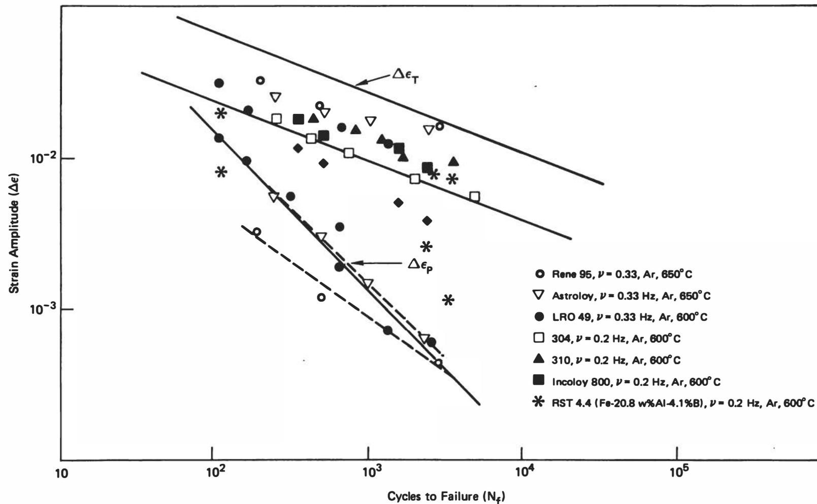
FIGURE 11 Low-cycle fatigue of ordered alloys compared to commercial alloys: Rene 95 ○ and Astroloy ▽ (unpublished material, S. V. Golwalkar, Rensselaer Polytechnic Institute); LRO 49 ● (unpublished material, A. K. Kuruville, Rensselaer Polytechnic Institute, 1983); 304 □, 310 ▲ and Incoloy 800 ■ (unpublished material, C. Zhi Ben, Rensselaer Polytechnic Institute, 1983); and RST 44 \* (Ray et al. 1983).
