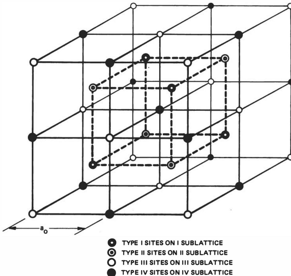
FIGURE 29 Generalized unit cell appropriate for description of  $DO_3$ ,  $L2_1$ , and  $B2$  superlattices. B atoms are confined to Type II sites for  $A_3B$  and  $DO_3$  structure and to Types I and II for  $AB$  with  $B2$  structure (Marcinkowski and Brown 1961).
