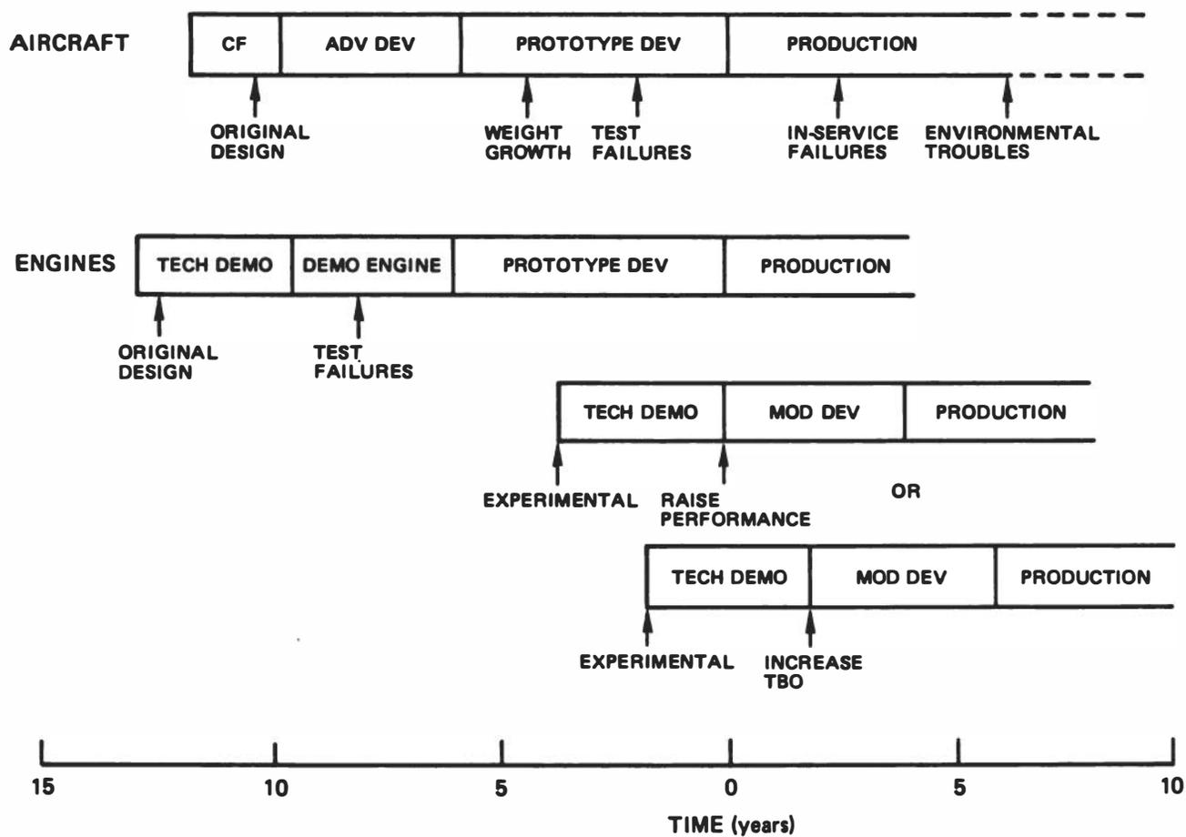
FIGURE 13 New material application windows (Ekvall et al. 1982).
