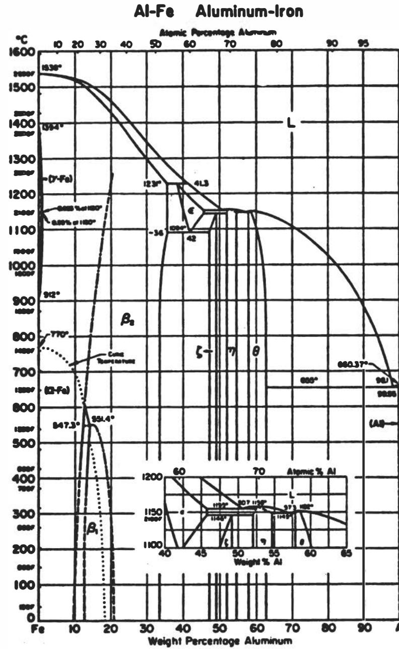
FIGURE 27 Fe-Al phase diagram (American Society for Metals 1973).
