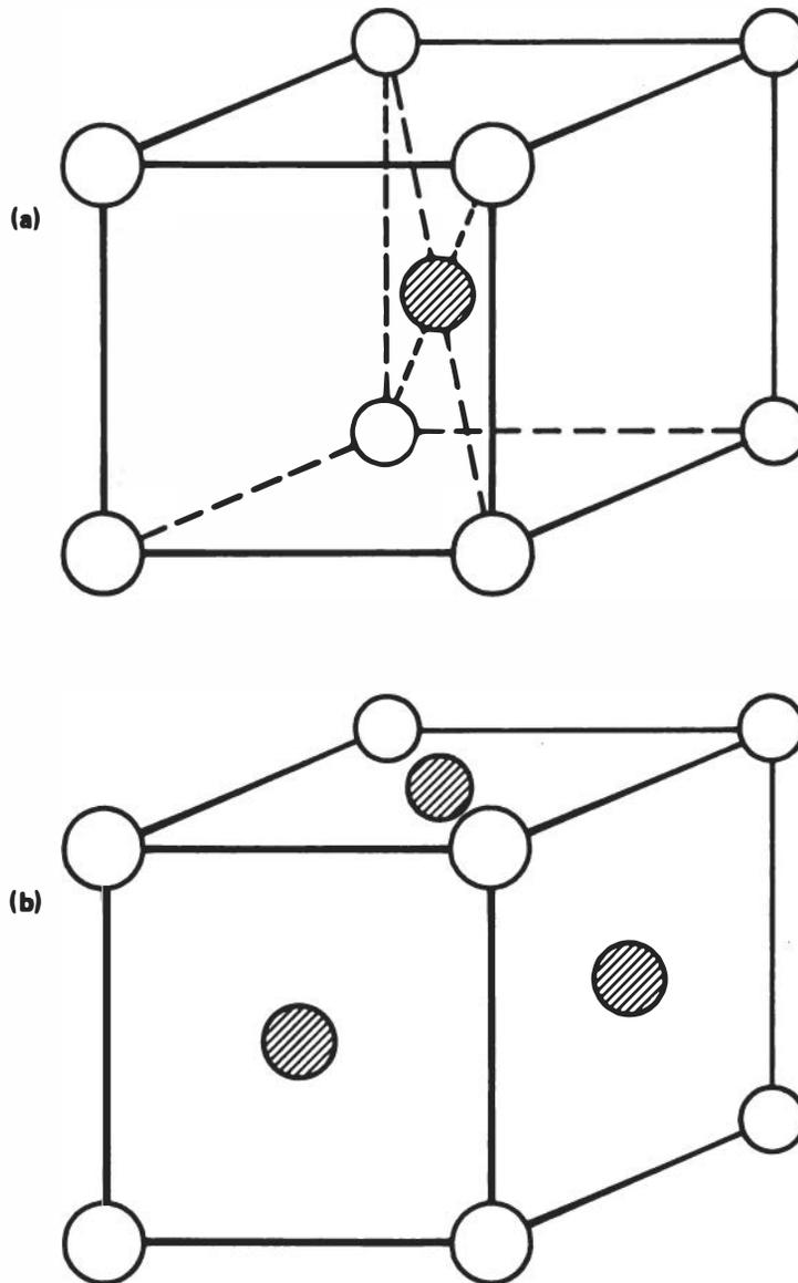
**FIGURE 1 (a) At low temperatures: CuZn has the cesium chloride B2 long-range-ordered structure and (b) Cu<sub>3</sub>Au has the face centered cubic-based L1<sub>2</sub> structure.**
