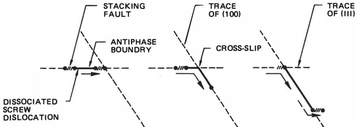
FIGURE 5 Cross slip of leading dissociated screw dislocations from (111) to (001), favored by lower APB energy on (001) (Kear and Wilsdorf 1962).
