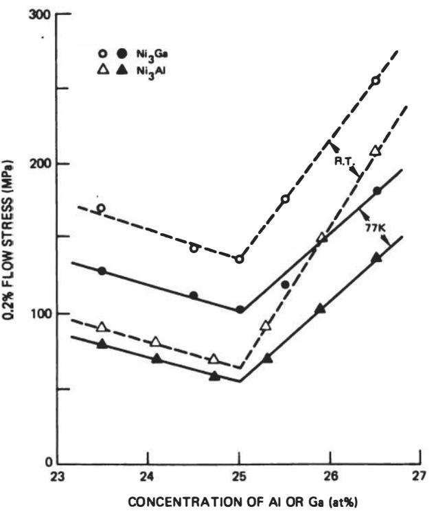
FIGURE 4 Effect of composition on the temperature dependence of yielding of binary Ni<sub>3</sub>Al alloys (Noguchi et al. 1981).
