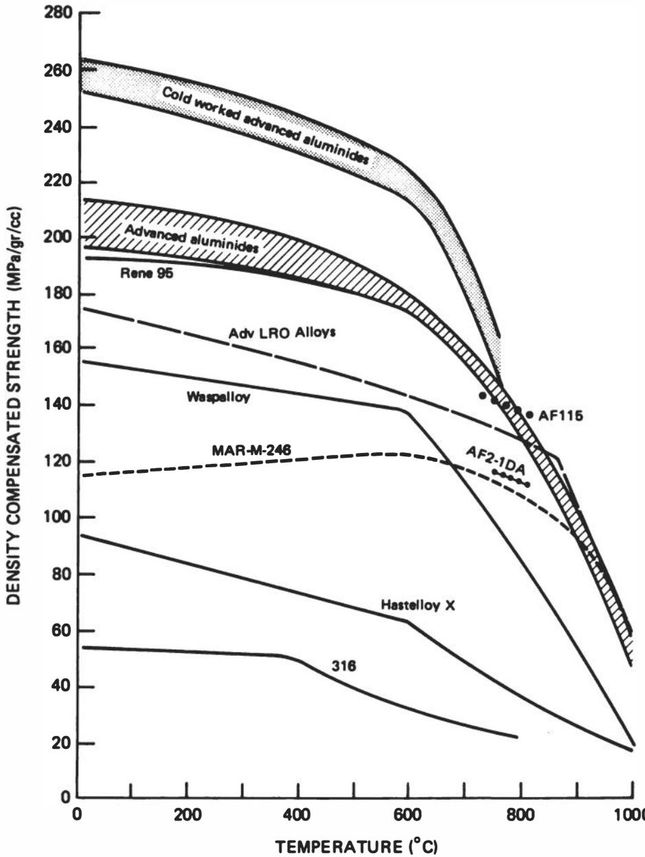
**FIGURE 25** Comparison of the density-compensated ultimate tensile strength of advanced LRO alloys and advanced nickel aluminides with commercial structural alloys.
