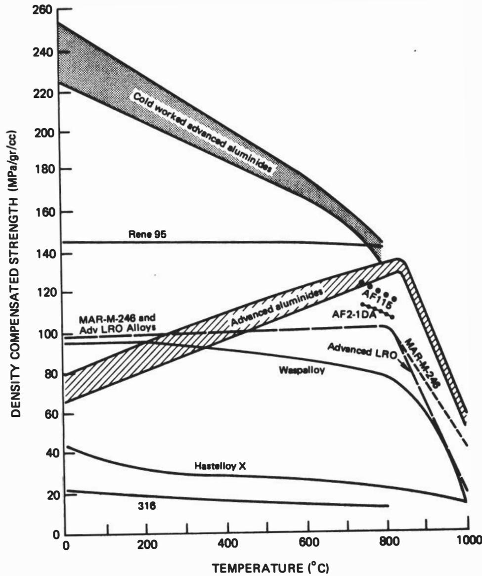
FIGURE 24 Comparison of the density-compensated yield strength of advanced LRO alloy and nickel aluminides with commercial structural alloys.
