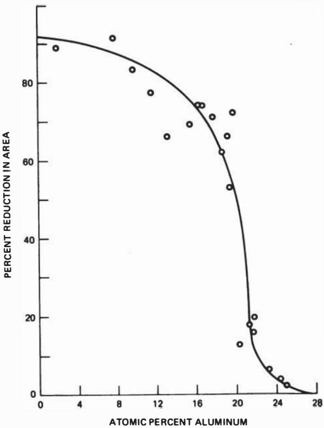
FIGURE 6 Ductility of Fe-Al alloys slowly cooled to 477°K and fractured in tension at that temperature (Marcinkowski et al. 1975).
