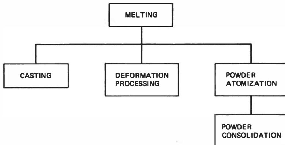
FIGURE 30 Current process routing for the production of ordered alloys.
