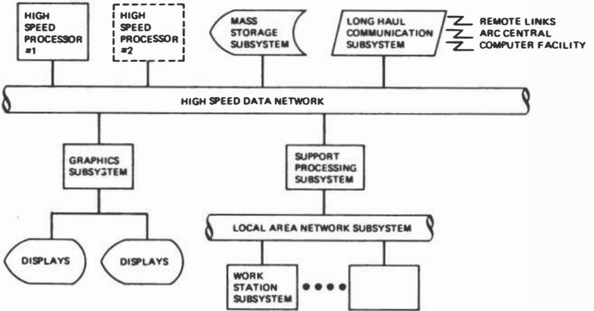
**Figure 2 The NAS Processing System Network (NPSN).
