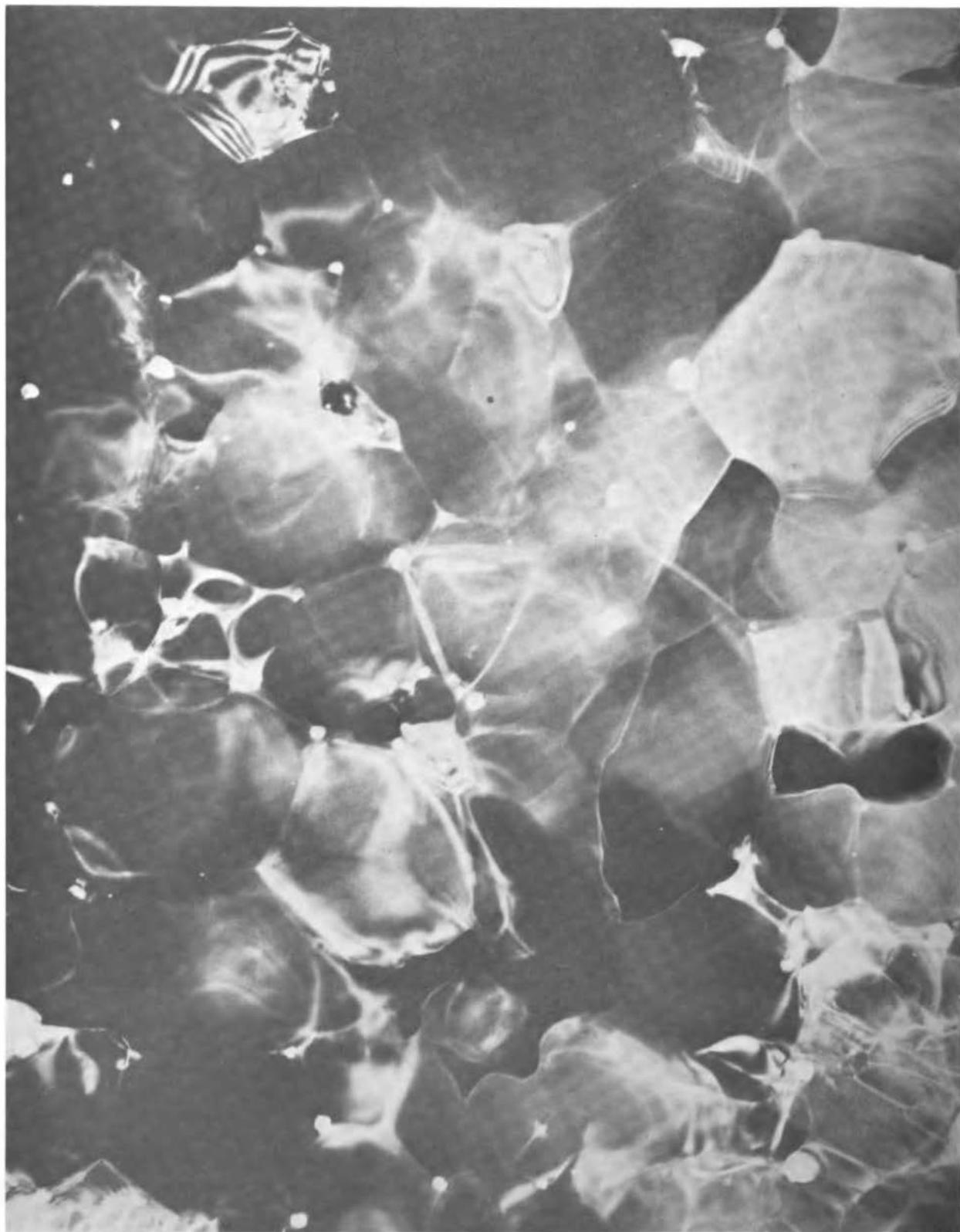
**FIGURE 31** TEM central core of explosively compacted AlN (Yust 1981)
