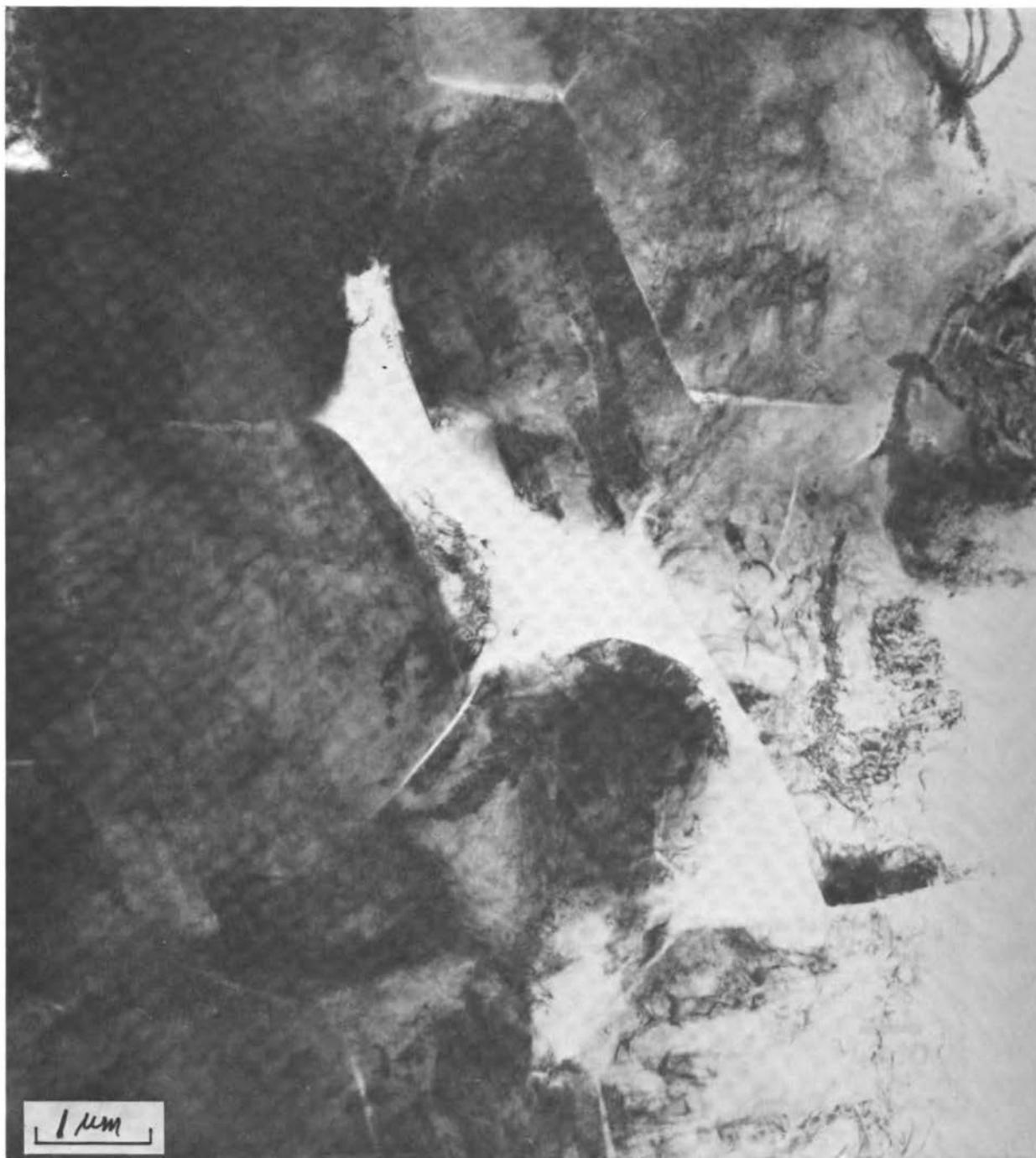
**FIGURE 18** Extensive plastic deformation in dynamically compacted alumina. Intense tangles of dislocations are visible within the individual grains, whose typical diameters will correspond to those of the starting material. Also note some local evidences of grain boundary sliding (displaced triple points), and cracking (Yust 1980)
