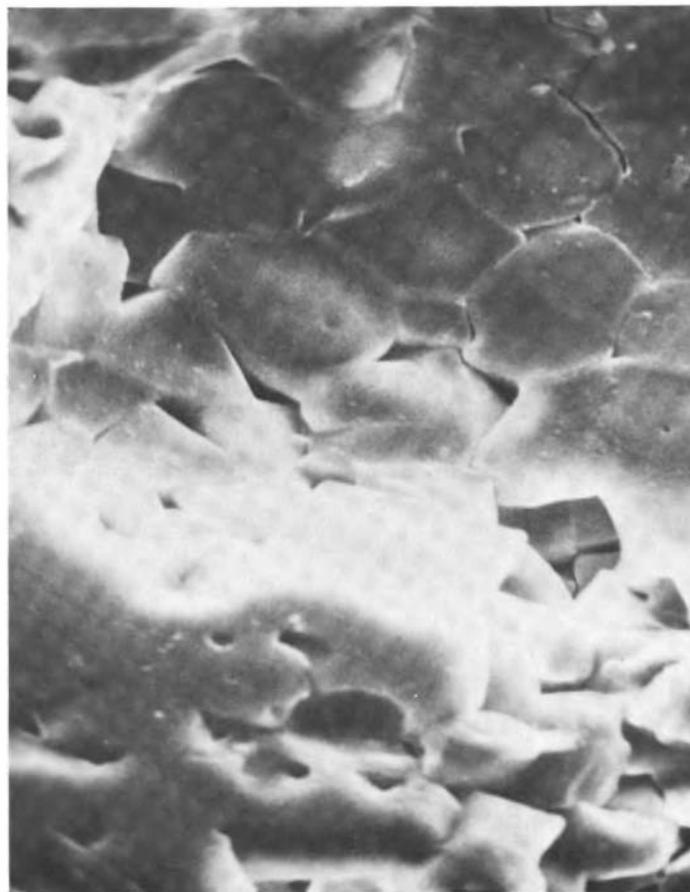
(b) Microstructural details at intersection of polished, thermally etched surface (lower portion) with large pore (upper portion) in Zone A, SEM X1750. Note 1) coarse and fine pore structures and 2) well-defined columnar grains at the solid-large pore interface.
