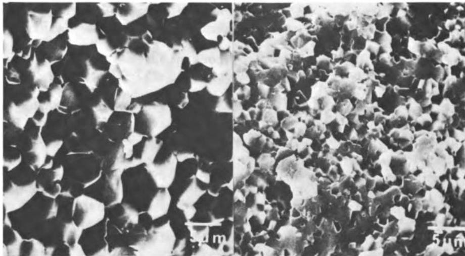
FIGURE 28 Microstructures in sintered alumina as functions of densification path (CTS, RCS), achieving same density ( $D = 0.99$ ) over same total densification time ( $t = 3 \pm 0.1$  hr): (a) CTS,  $1530^{\circ}\text{C}$ , 2 hr soak; (b) RCS, peak temperature  $\sim 1560^{\circ}\text{C}$ , no soak. Note: typical grain size ranges: CTS  $1.8\text{--}5.2 \mu\text{m}$ ; RCS  $1.2\text{--}2.8 \mu\text{m}$  (Palmour, Huckabee, and Hare 1977)
