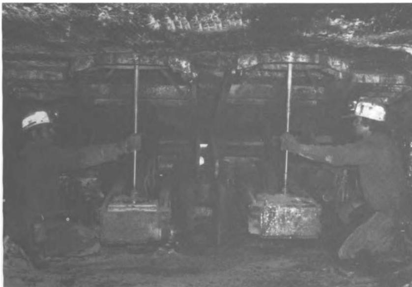
FIGURE 5 A Lee-Norse TD-2 roof bolter with automated temporary roof support (ATRS) in use at the Homer City Mine in Pennsylvania.
