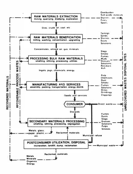
FIGURE 1 Materials supply, utilization, and disposal sections.
