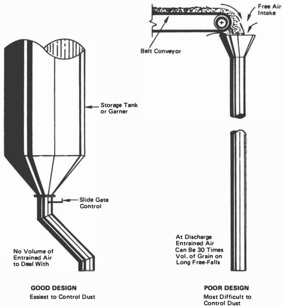
FIGURE 6-11 Load-out spout design.
