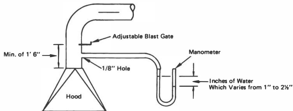
FIGURE 8-3 Typical hood and blast gate.
