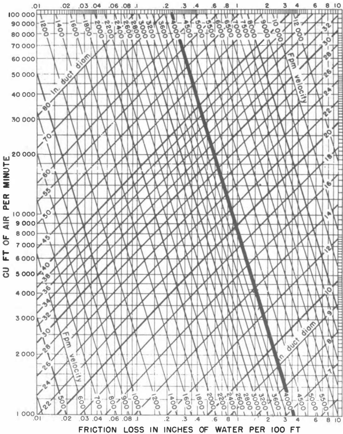
(Based on Standard Air of 0.075 lb per cu ft density flowing through average, clean, round, galvanized metal ducts having approximately 40 joints per 100 ft.)
