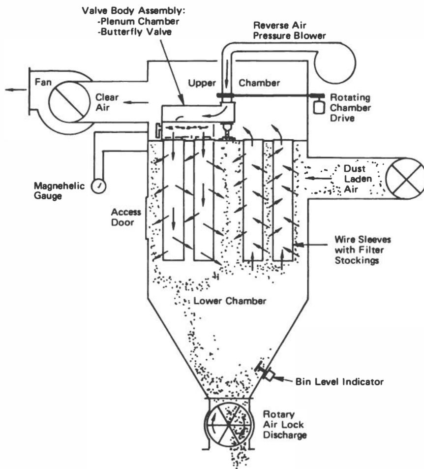
FIGURE 4-1 Typical fabric filter.
