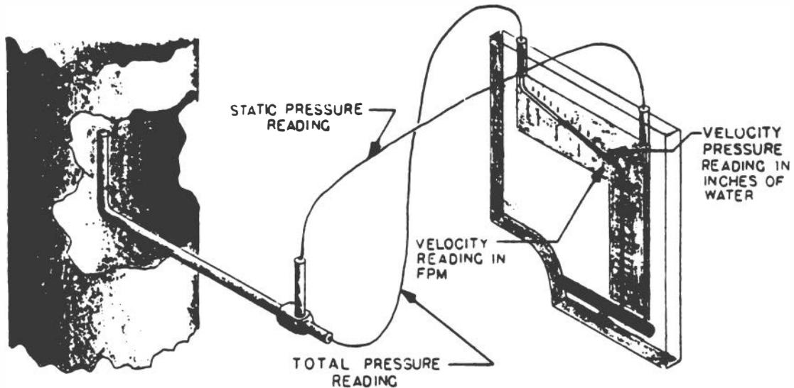
FIGURE C-4 Use of pitot tube and velometer.
