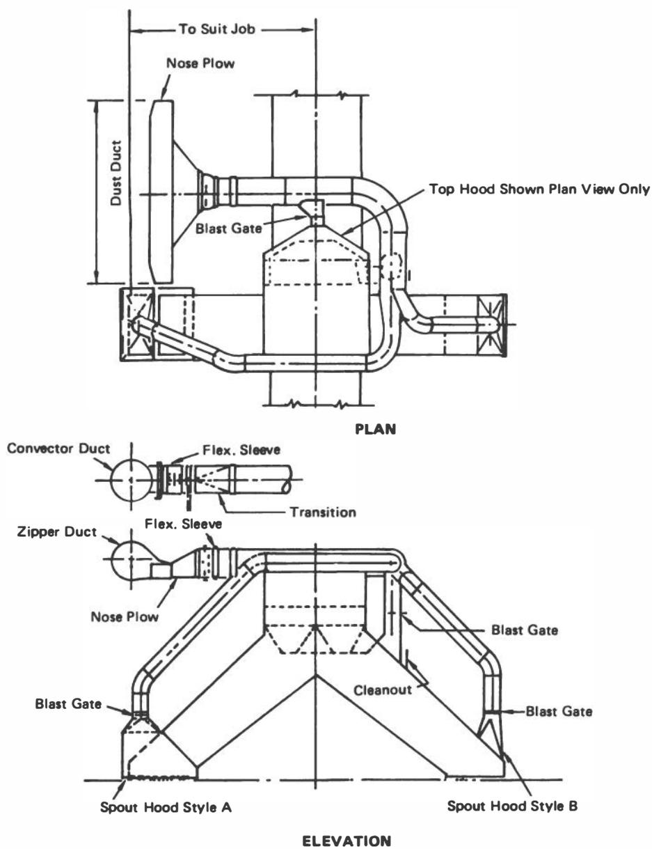
FIGURE 6-7 Zipper suction for tripper.
