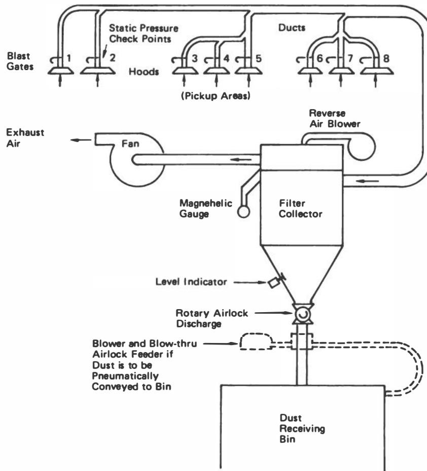
FIGURE 8-1 Typical dust control system. The figure shows an exhaust system because the fan draws air through the collector. If the fan is ahead (i.e., pushing air through) of the collector, it is a blow system. Most cyclone collectors are attached to blowing systems, and most filter collectors are attached to exhausting systems.
