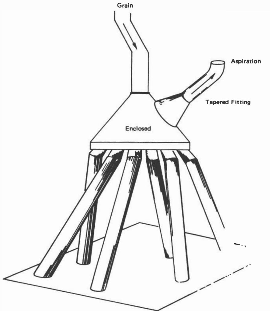
FIGURE 6-6 Enclosed distributor dust control system.
