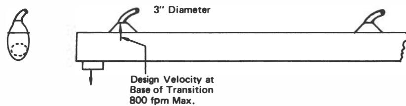
NOTES: Cover must be complete and tight. Add additional take-offs to remove displaced air,  $\text{cfm} = \text{bpm} \times 1.25$ . Makeup air inlets may be required when the system is airtight.
