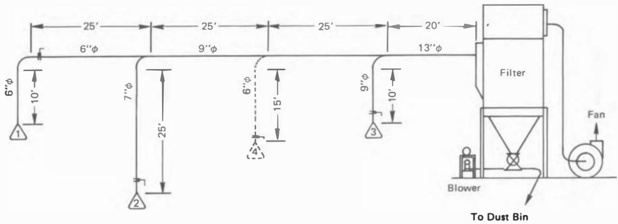
FIGURE 3-5 Typical dust-collection system.
