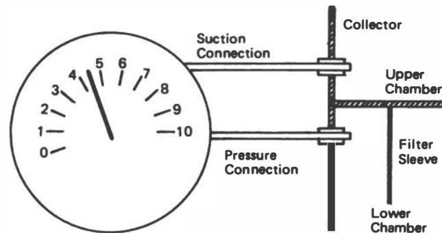
**FIGURE 8-2** Typical magnehelic gauge installation. The best method of determining whether a collector is operating effectively is to check the magnehelic gauge. If filter resistance is above 3-4 inches of static pressure (SP difference between the upper and lower chamber), check the filters for excessive dust accumulation.
