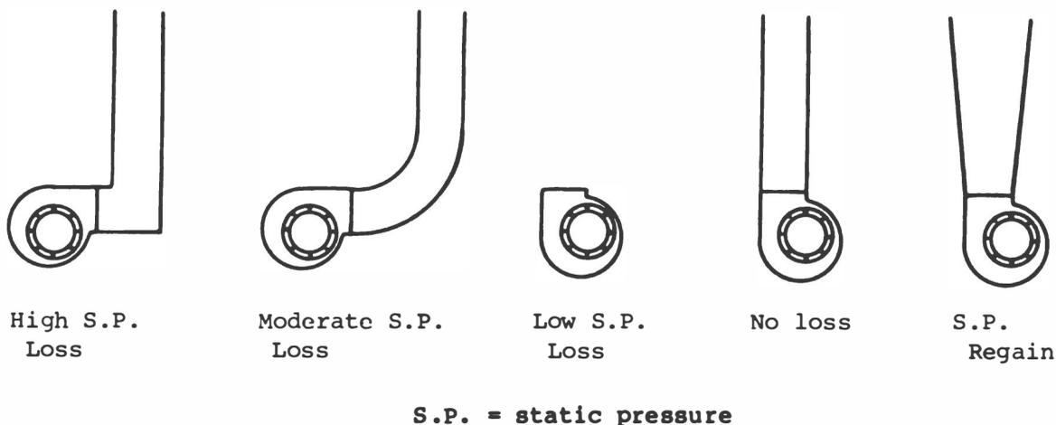
FIGURE 5-7 Effects of fan discharge methods upon static pressure.
