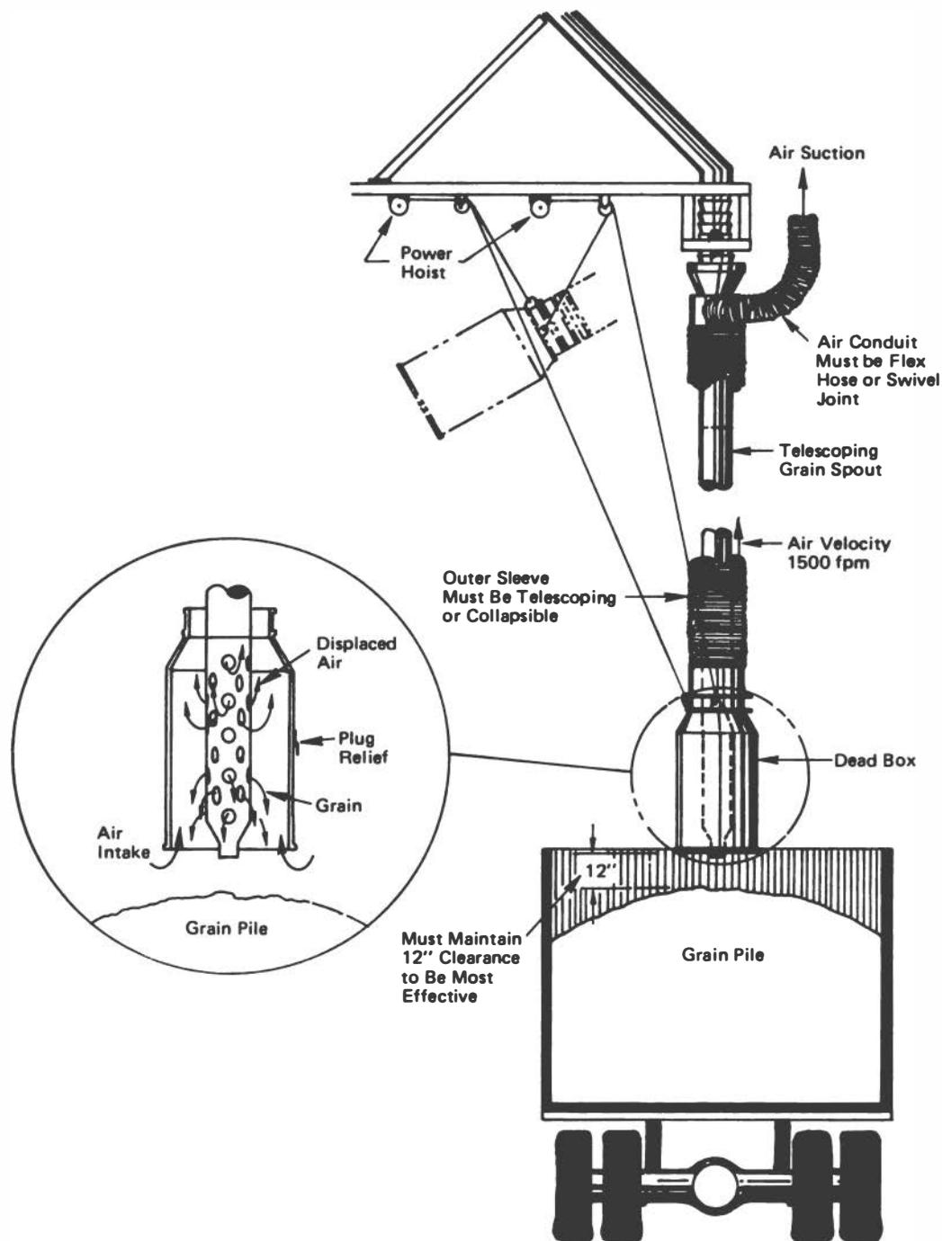
FIGURE 6-9 Retractable spout deadbox for truck load-out.
