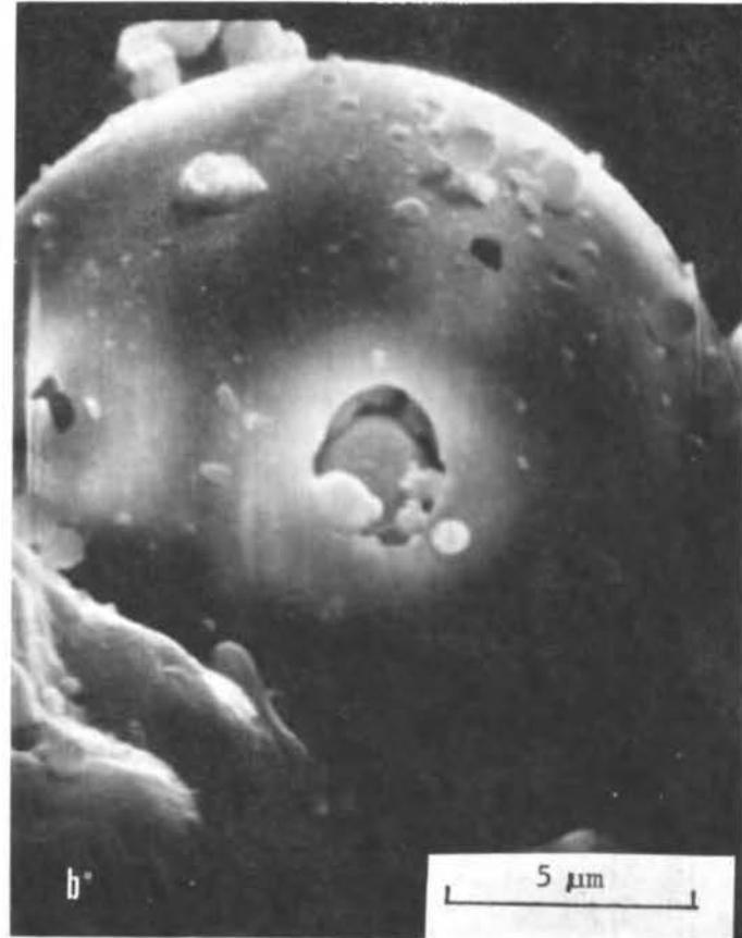
**FIGURE 13** Plerosphere with submicrometer spherical inclusions and attached surface spheres: (a) 2000 $\times$ , (b) 6000 $\times$  (Page et al., 1979).
