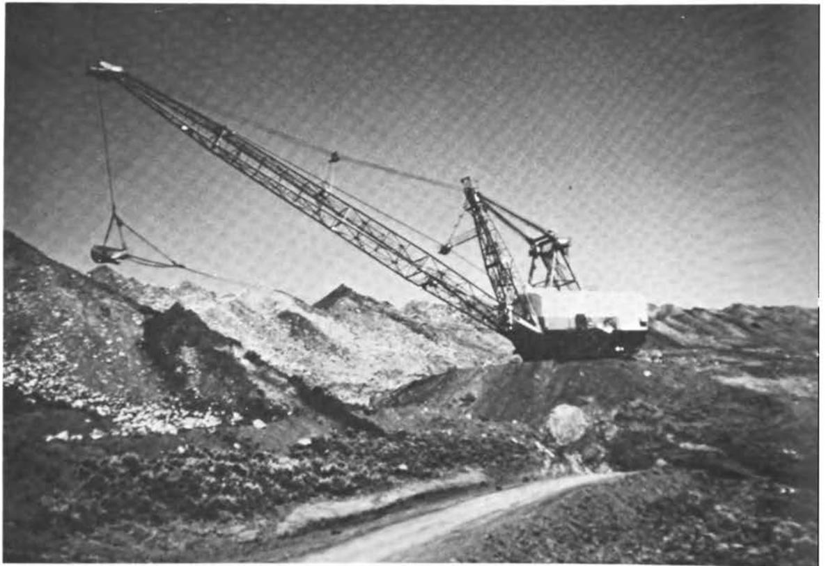
FIGURE 10 Dragline on an interburden bench casting spoil to its right.
