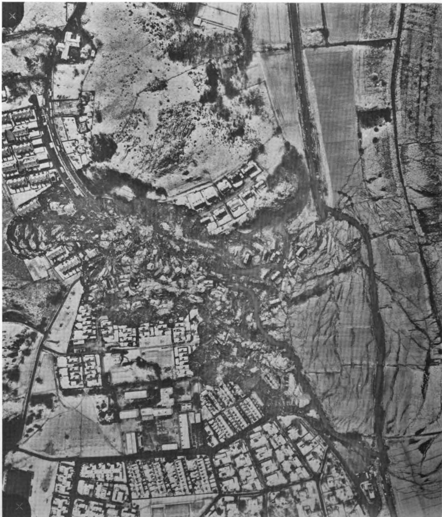
Fig. 4 Air photo of the Tuve region after the landslide of November 30, 1977.
