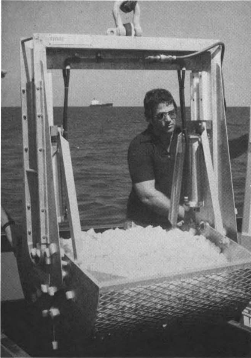
Figure 31 Recovered chips being removed from well by clamshell
