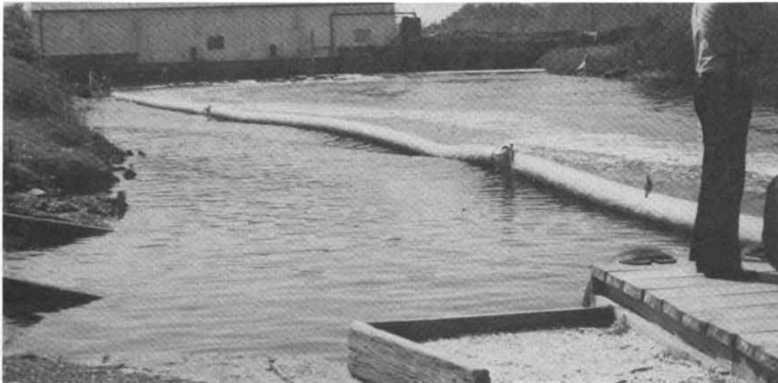
Figure 6 Fully extended boom showing wave conformance characteristics
