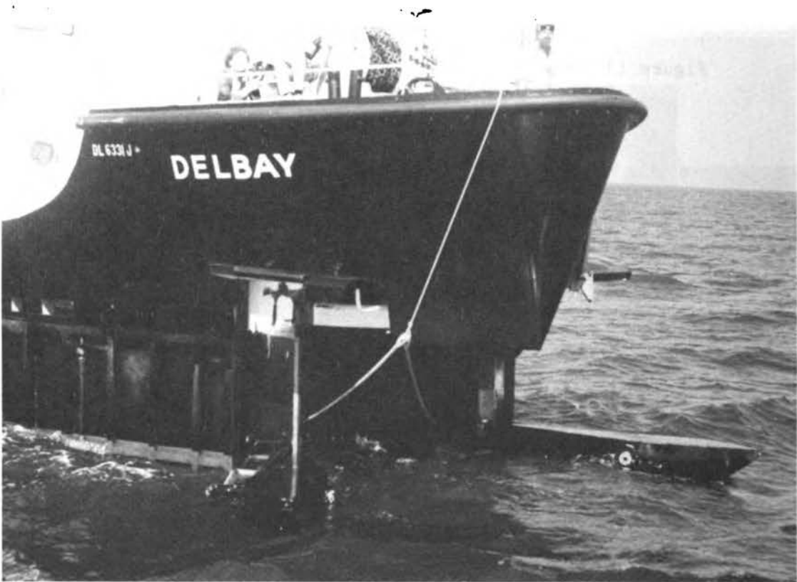
Figure 16 View of sweeps and opening to collection system
