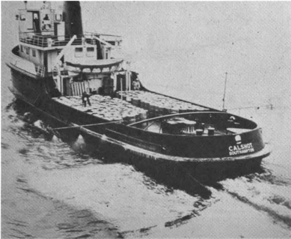
Figure 36 Dispersant spraying through booms followed by breaker-board mixing
