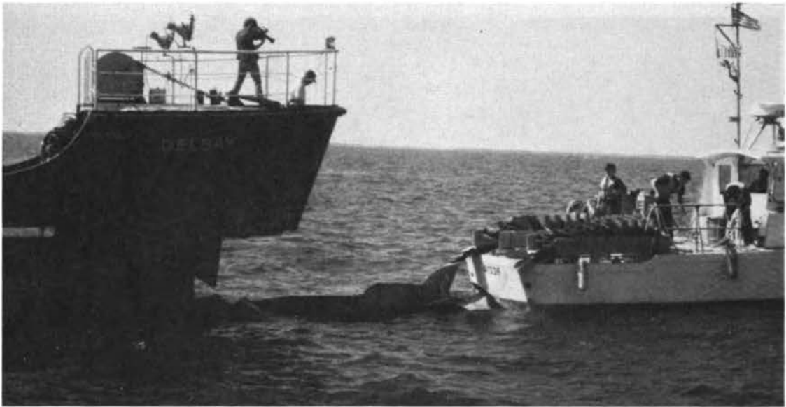
Figure 19 Beginning of boom deployment for V-configuration
