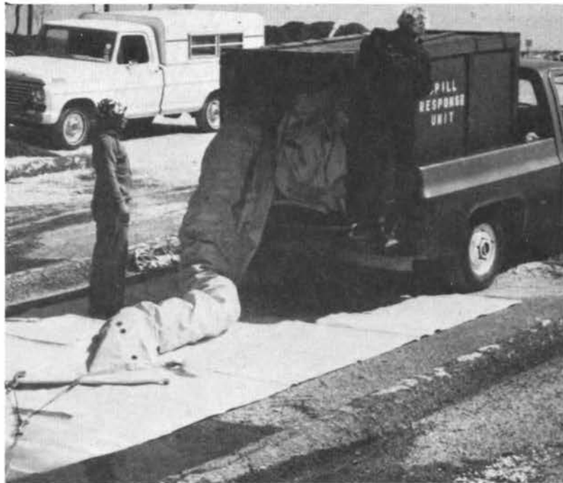
Figure 3 Initiation of boom deployment
