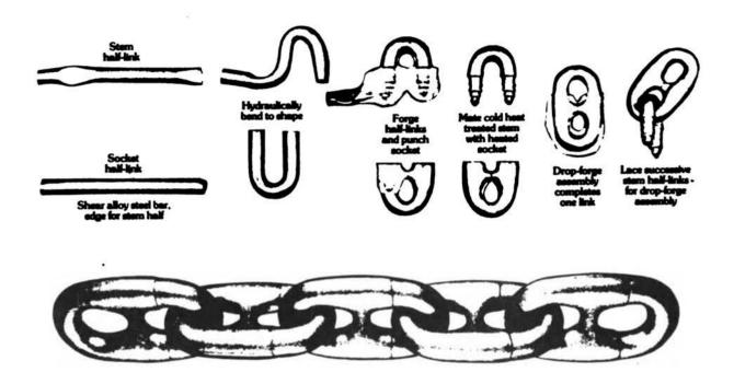
FIGURE 1 Processing Steps for Forging Die Lock Steel Stud-Link Anchor Chain. From CASREPT, 1979.
