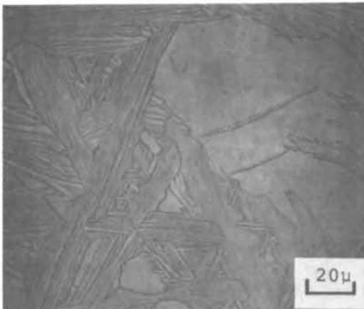
Figure 3. Widmanstätten or transformed beta Ti-6242 microstructure
