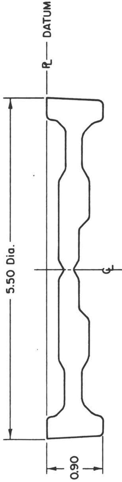
Figure 12. Subscale compressor disk forging
