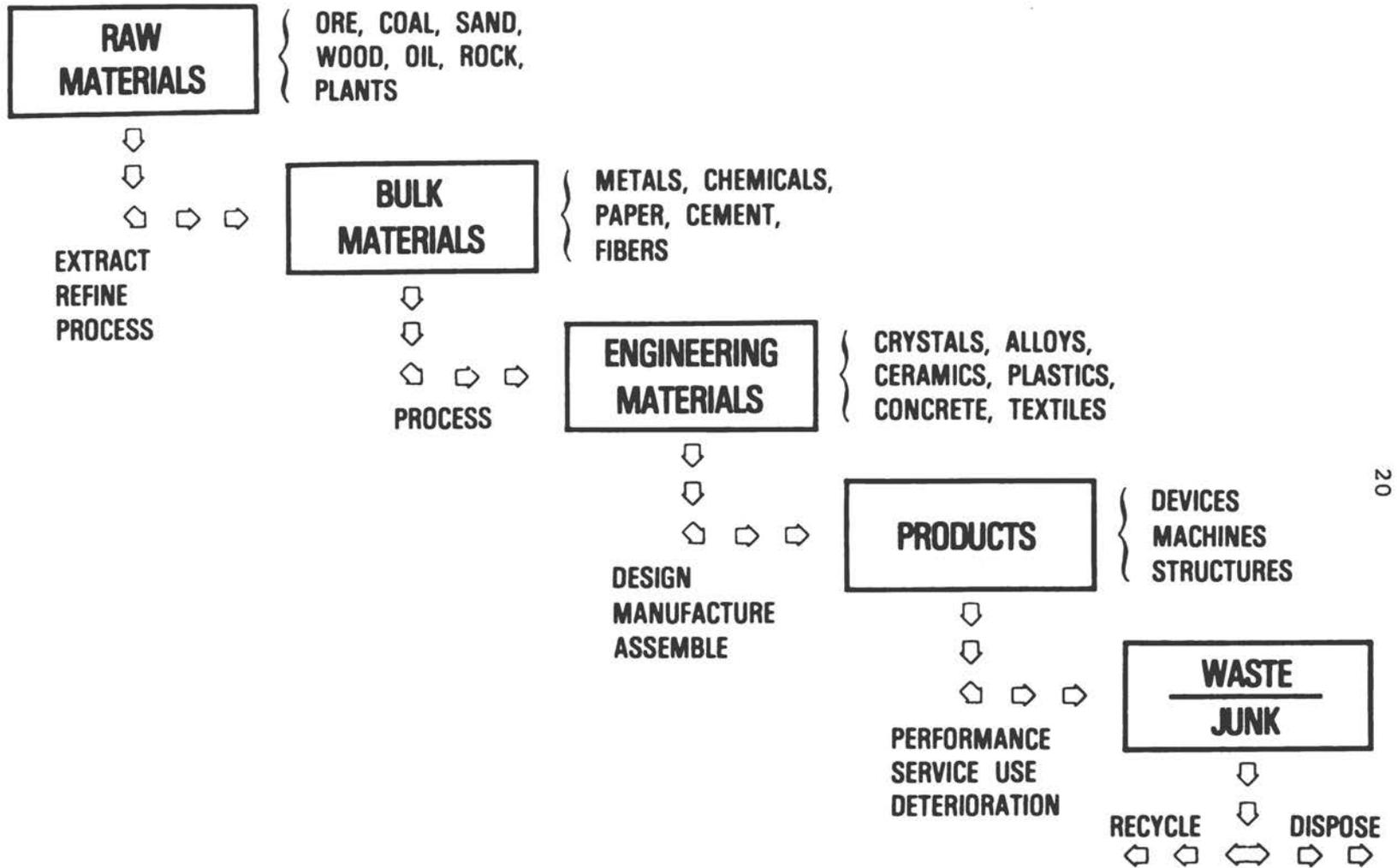
Figure 3. Materials and processing sequence
