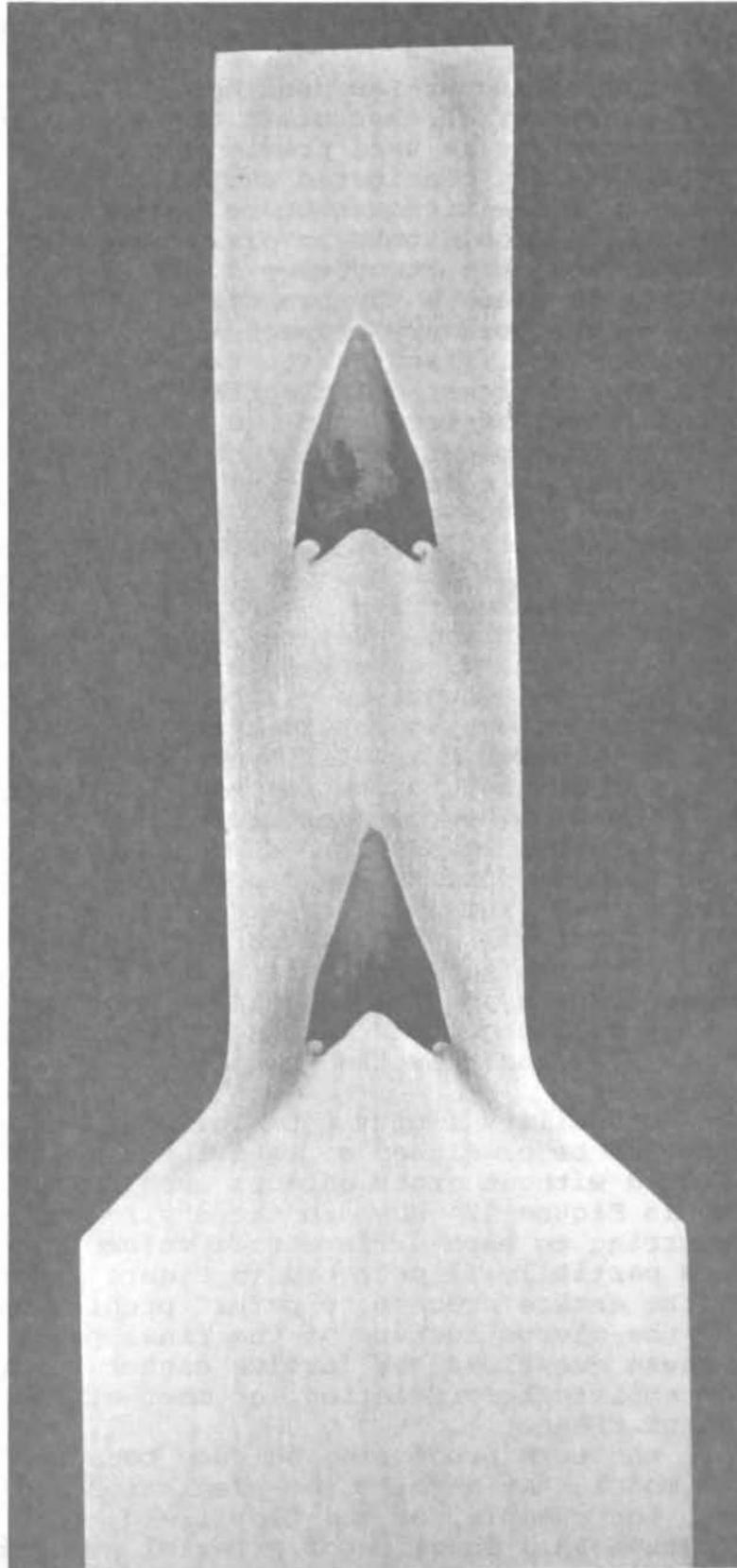
Figure 1. Illustration of central burst fracture during extrusion
