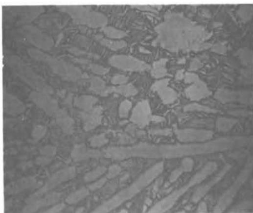
Figure 4. Primary alpha plus transformed beta Ti-6242 microstructure
