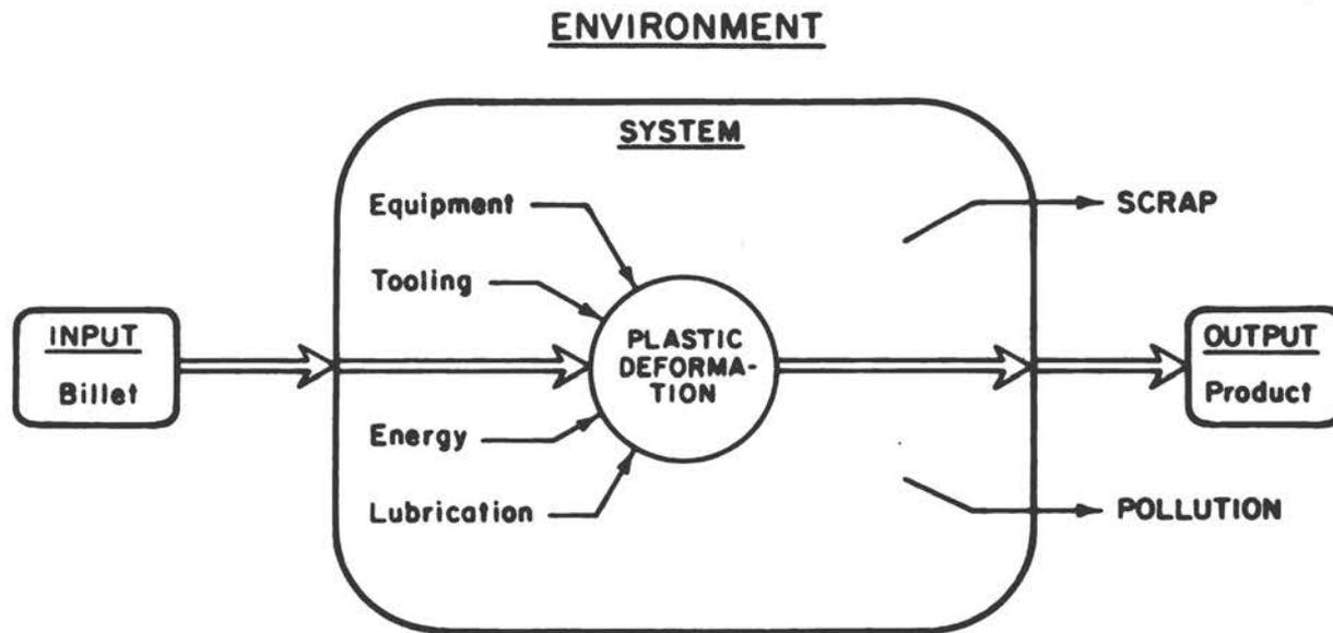
Figure 2. Deformation process as a system
