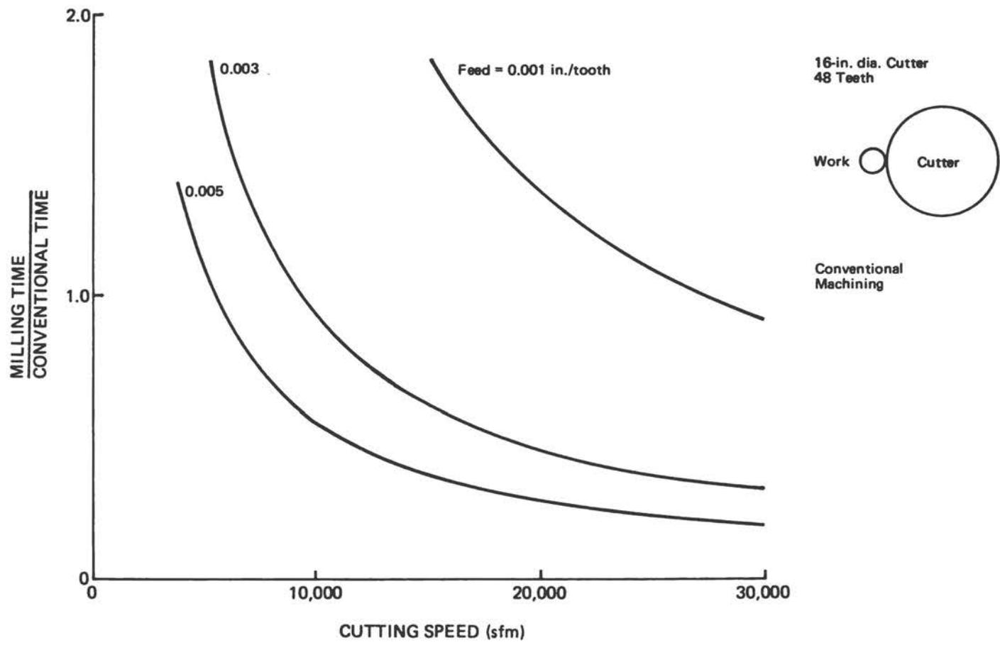
Figure 3. Effect of cutting speed on the ratio of milling time to conventional time as a function of feed/tooth for machining a steel automotive reverse sun transmission gear
