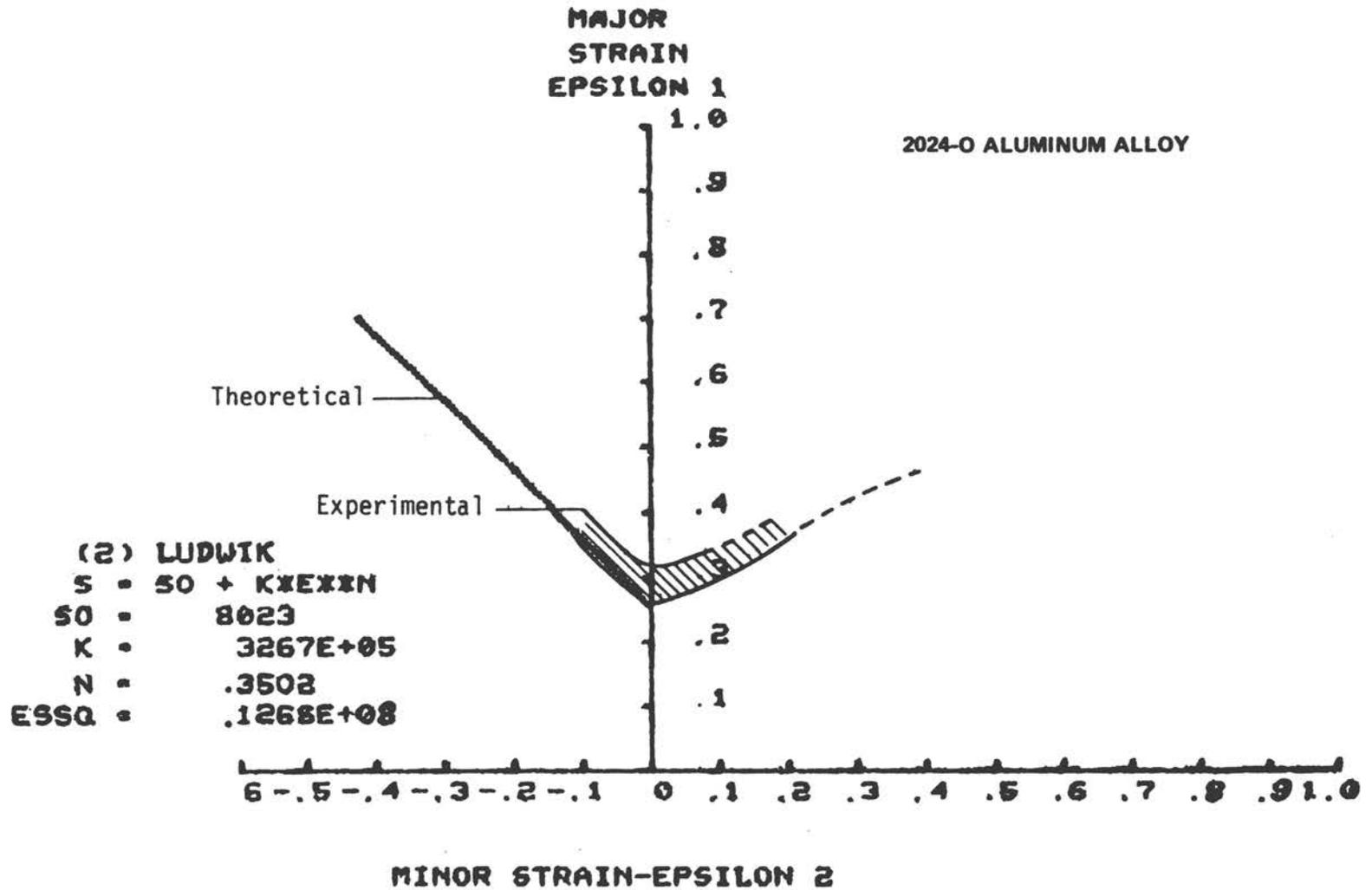
Figure 6. Comparison of theoretical forming limit curve with experimental curve
