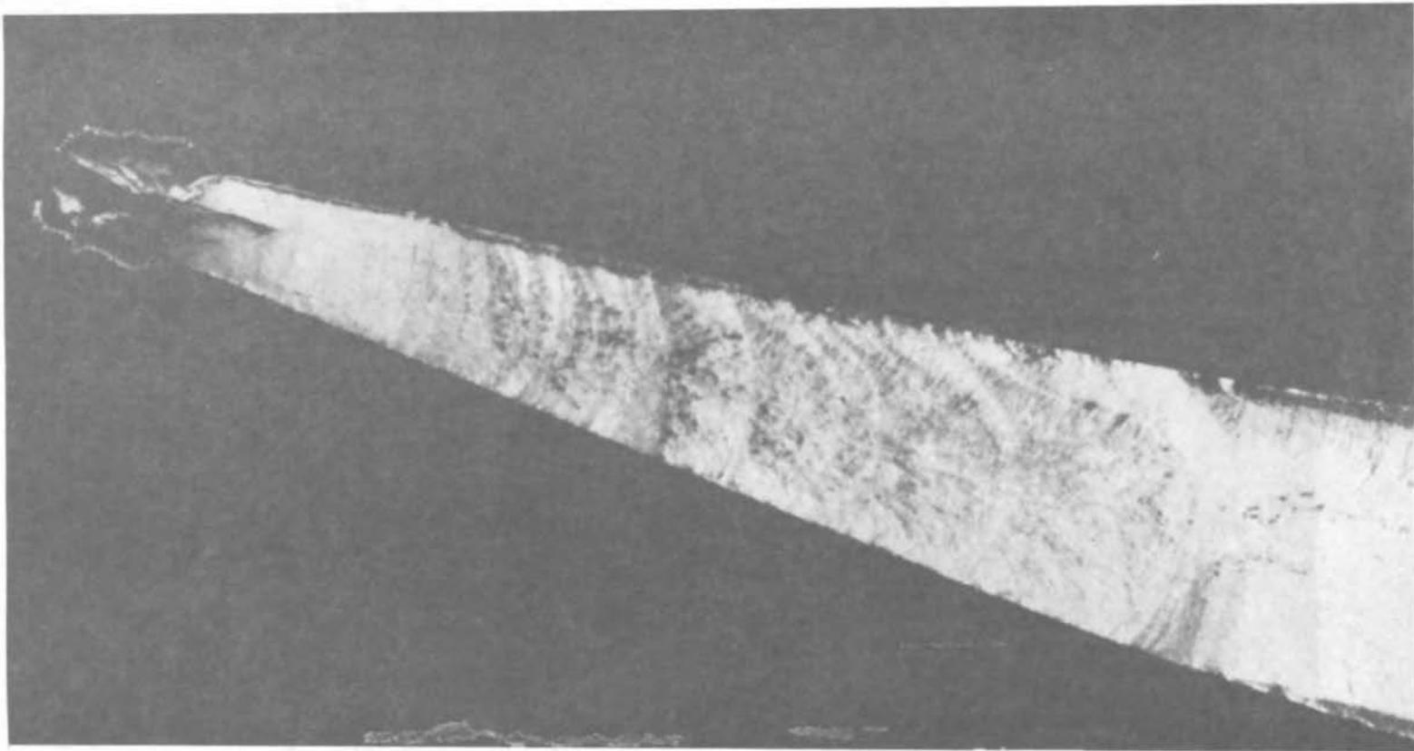
Figure 10. Shear band defect caused by die chilling leading to a fatigue failure
