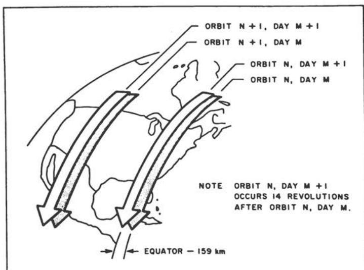
FIGURE 20 Landsat orbits repeat on an 18-day cycle. Adjacent swaths on adjacent days overlap some 15 percent near the equator; the overlapping becomes progressively larger at higher latitudes.
