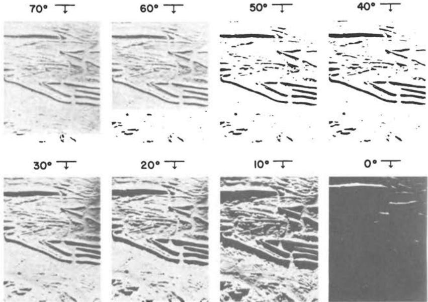
FIGURE 25 Differential emphasis of geologic and topographic structures is shown by different angles of solar or radar illumination. This model simulates both. It is clear that subtle topographic and geologic features need shallow angles of illumination, whereas major structural features would still be identifiable with steeper illumination angles.
