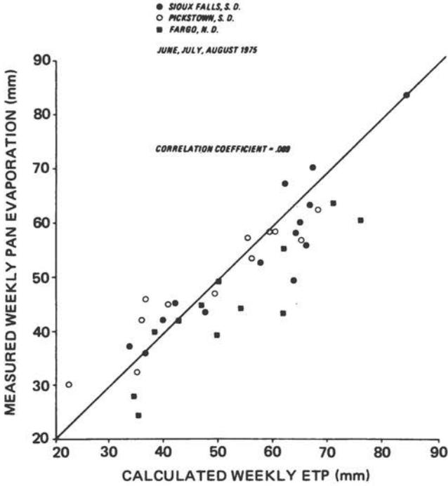
FIGURE 26 Comparison of weekly measured pan evaporation and evapotranspiration calculated by the Earth Satellite Corporation computer program known as METRUN during June, July, and August 1975 for Fargo, North Dakota, and Sioux Falls and Pickstown, South Dakota.
