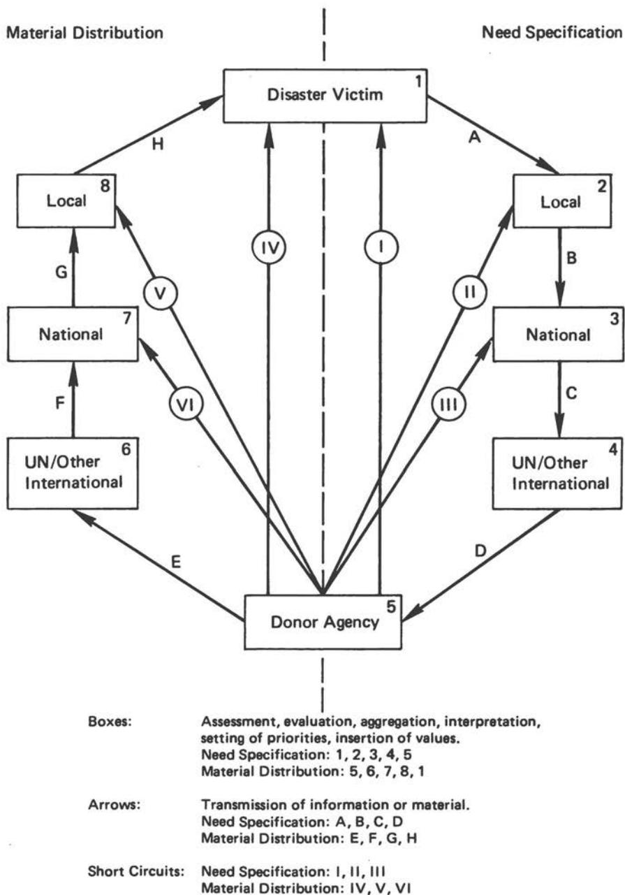
FIGURE 19 Simplified diagram of need specification and relief distribution.
