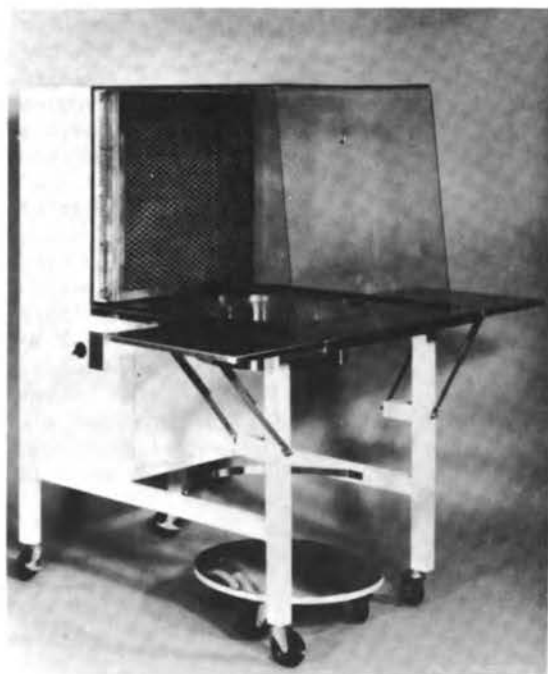
FIGURE 5 Portable unit for disposing of animal bedding, with negative flow of air through the canopy portion of the cabinet.
