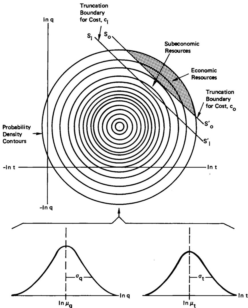
Note:  $q$  = deposit average grade;  $t$  = deposit tonnage.
