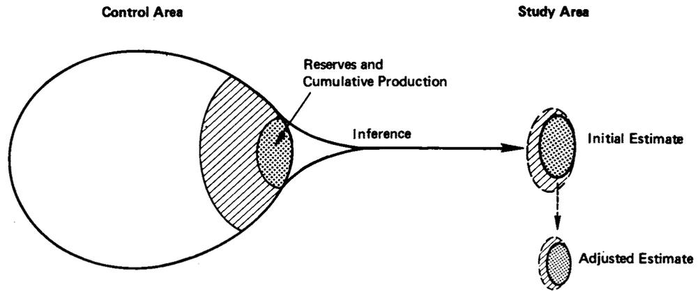
FIGURE 4.2 Estimation of potential supply by geologic analogy.
