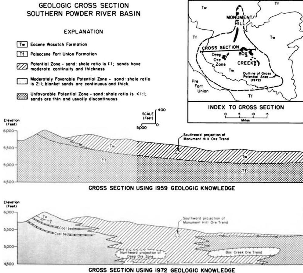
FIGURE 1.3 Generalized geologic cross sections of Powder River Basin, Wyoming, illustrating 1959 and 1972 geologic knowledge.
