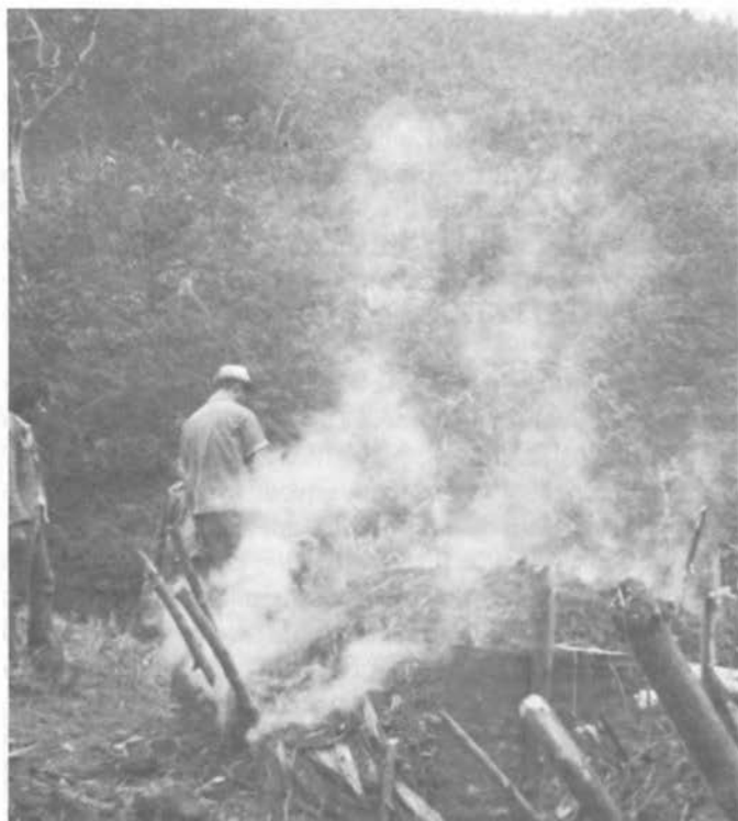
FIGURE 33 Mabuhay Vinyl Corporation, Mindanao, Philippines. Trial charcoaling of leucaena wood for the production of calcium carbide and vinyl plastics. This use of leucaena may offer a way to convert eroding tropical wastelands to productive use. It is suitable for large- or small-scale enterprises that can provide jobs and income in rural regions. In the background, leucaena covers slopes that, 18 months before, were bare, eroding, limestone soils. In that short time many of the trees have grown to over 7 m tall. (M. D. Bengé)
