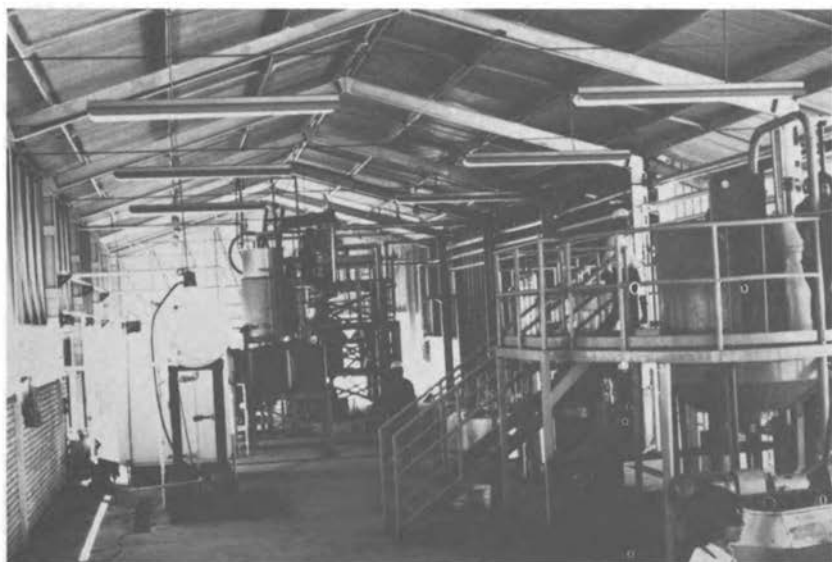
Figure 17. A section of the Government of Mexico's pilot guayule-processing mill at Saltillo, Coahila. Scaled to handle 1 ton of shrub daily, the facility has been constructed to optimize the processing methods developed in recent years by Mexican researchers. Current plans call for scaling up to large production (300,000 tons of shrub per year) by 1979. On the right are seen parts of the Bauer mill and flotation vats; in the background is the unit for removing resins from the crude rubber. (N. D. Vietmeyer)
