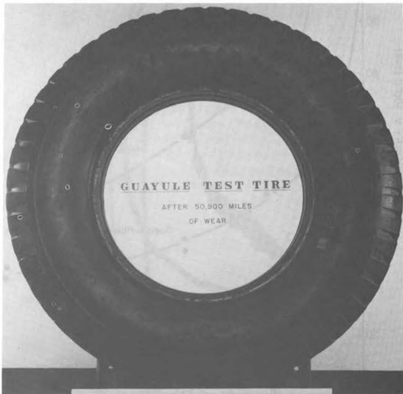
Figure 27. This—the first successful truck tire ever built of guayule rubber—was made from rubber grown and processed by the U.S. Natural Rubber Research Station, Salinas, California. Carcass construction is 100 percent guayule rubber with tread made of synthetic rubber. Road tests, in which the tire was run continuously at 45 mph with approximately 40 percent overload, were made by the Office of Rubber Reserve, Camp Bullis, Texas. Guayule proved to be the equal of hevea rubber in these tests. This tire, one of a test lot, was fabricated in 1953 by the Firestone Tire and Rubber Company, Akron, Ohio. (U.S. Department of Agriculture)
