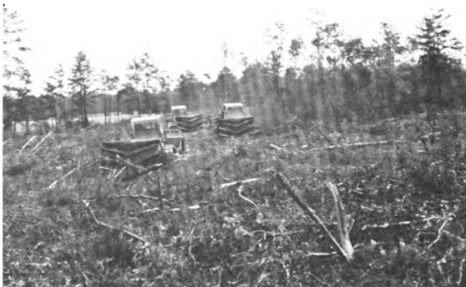
FIGURE 12. Mechanical site treatment with crawler tractors and rolling drum choppers in preparation for prescribed burning to provide site conditions suitable for establishing new stands of southern pine.
