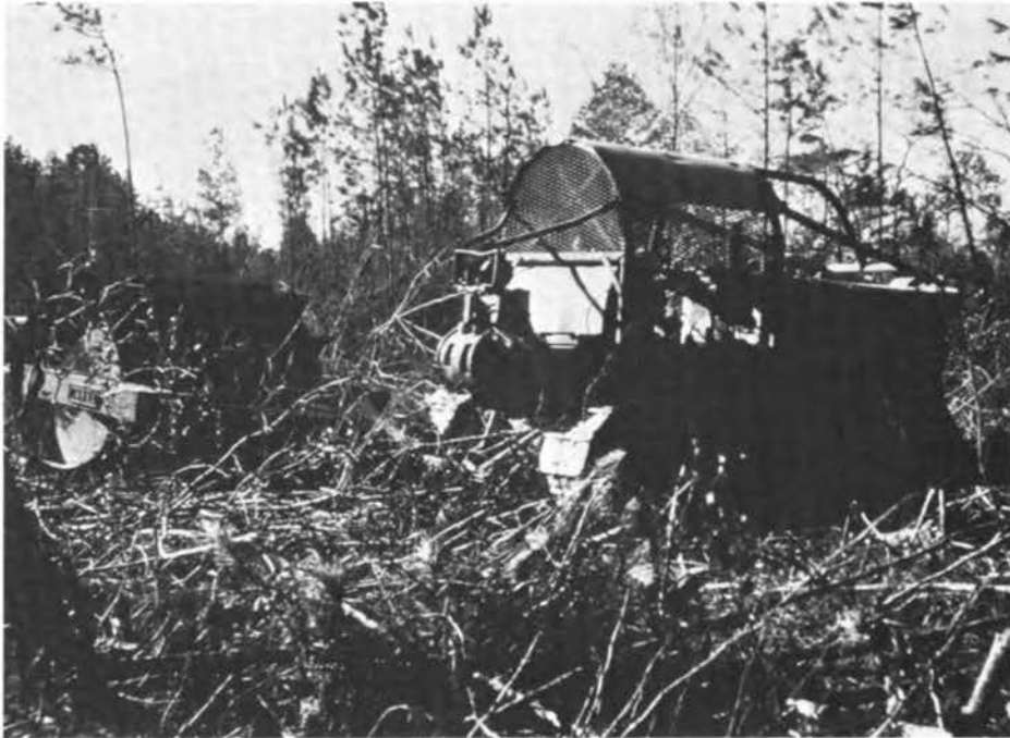
FIGURE 11. Mechanical site treatment with crawler tractors and rolling drum choppers in preparation for prescribed burning to provide site conditions suitable for establishing new stands of southern pine.
