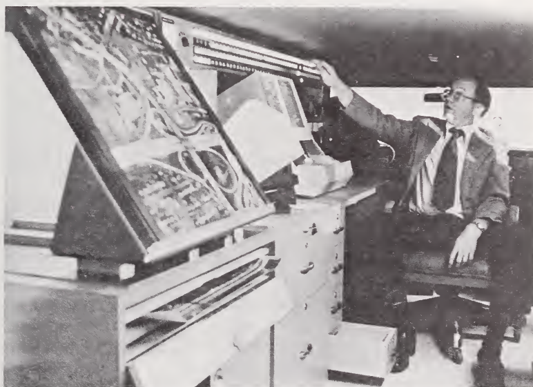
FIGURE 22 Internal view of mobile command and control van showing aerial photo board and equipment status board, looking from back to front of the van.
