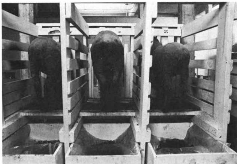
FIGURE 4 Wooden metabolism crate for sheep. (Courtesy of M. E. McCullough, University of Georgia Agricultural Experiment Stations)
