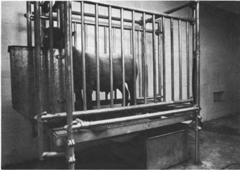
FIGURE 1 Metal metabolism crate for sheep (side A). (Courtesy of M. E. McCullough, University of Georgia Agricultural Experiment Stations)
