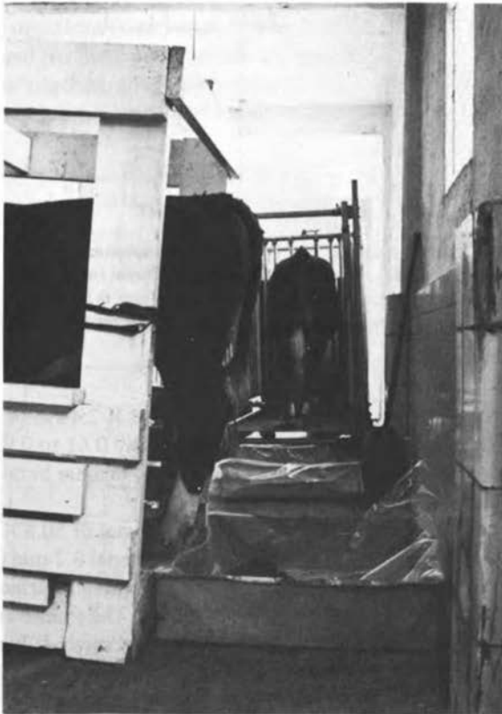
FIGURE 5 Metabolism stall for steers. (Courtesy of M. E. McCullough, University of Georgia Agricultural Experiment Stations)
