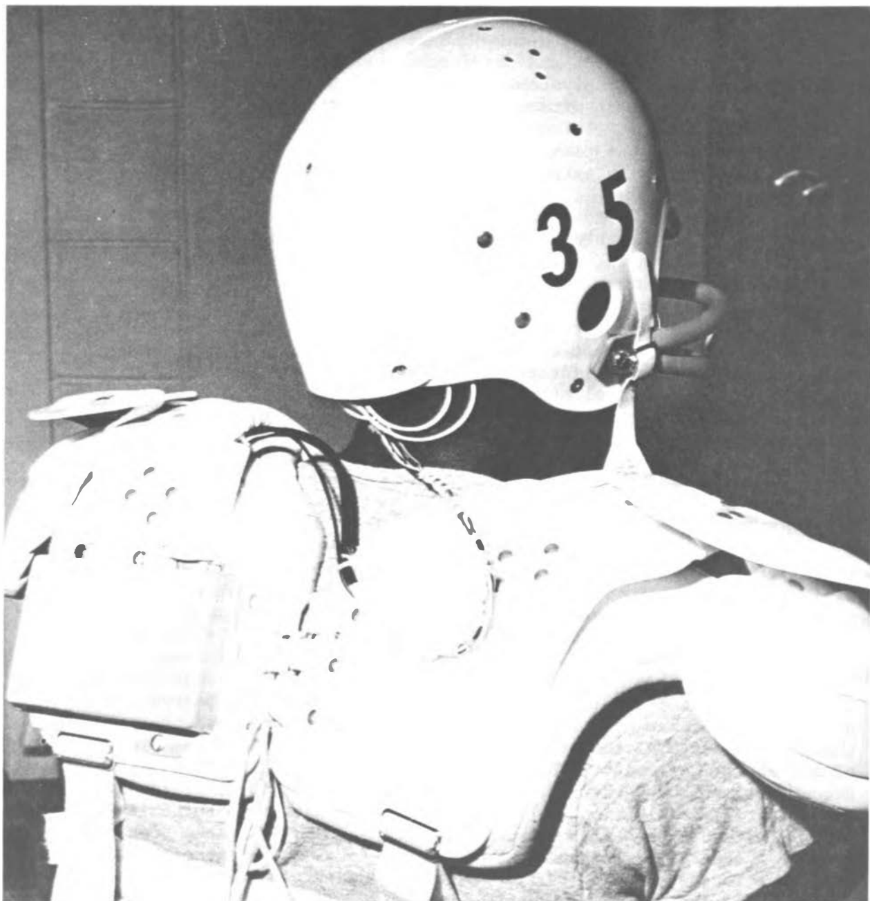
FIGURE 5 Woody Campbell with EEG transmitter compartment on helmet and radio station on shoulder pads for telemetering impact.
