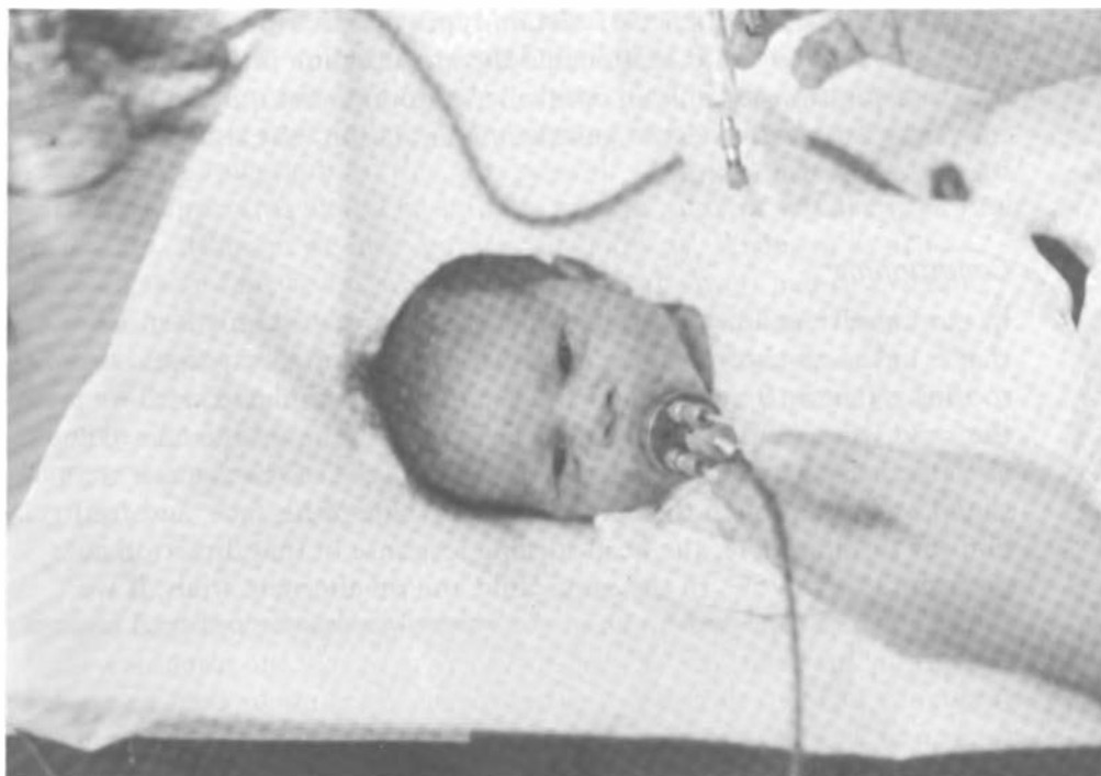
FIGURE 2 Newborn infant sucking on automatic nipple device that enables polygraphic recording of suction. Three wells surrounding the transducer enable administration of different nutrients or tastes.
