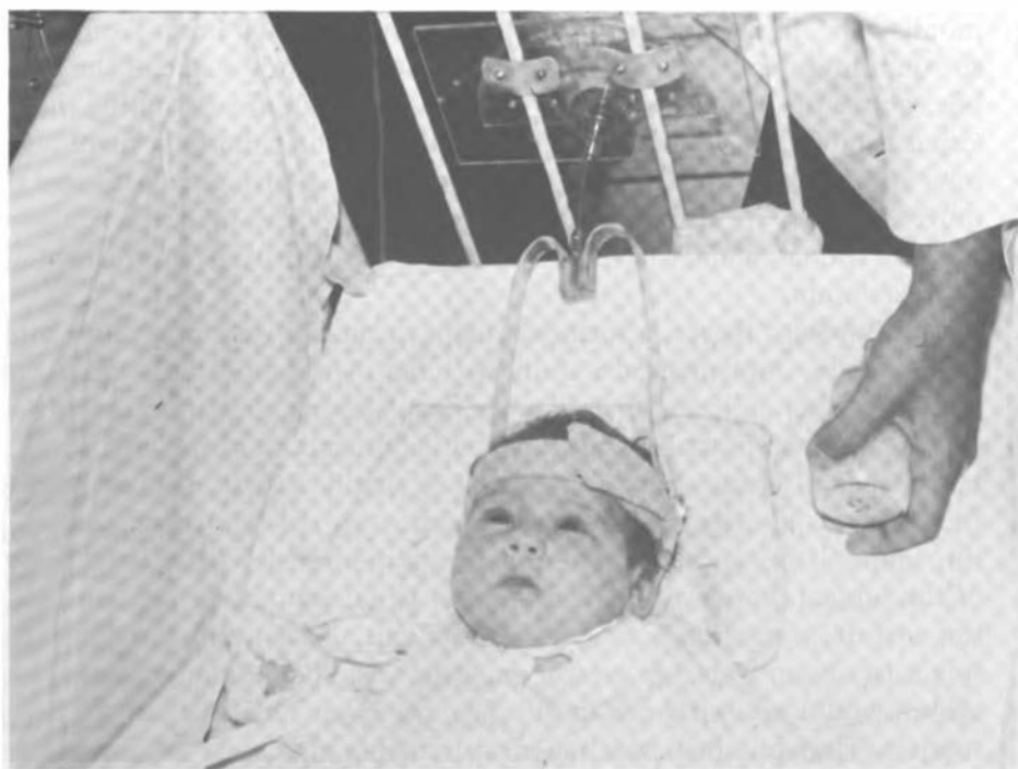
FIGURE 3 Infant attached to apparatus for recording head-turning. The plastic yoke is attached to a rotary potentiometer allowing polygraphic recording of incidence and magnitude of head-turning activity.
