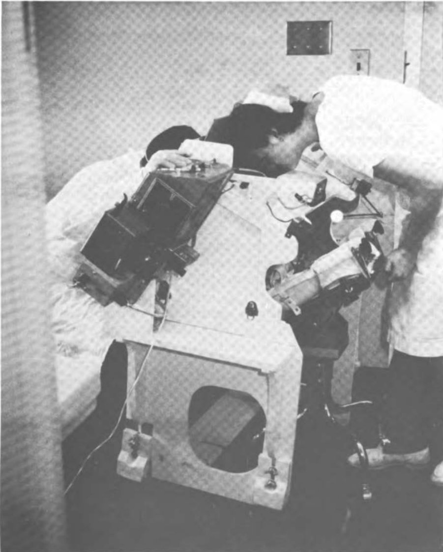
FIGURE 1 Visual-preference testing apparatus in mock operation. So that the baby could be seen in the picture, the crib was not set in as far as it would be in normal operation. The experimenter observes through a peephole between the targets. The second observer (standing) looks at a mirror above this hole. The recording unit and timer can be seen in the foreground. (From Miranda. 26 )
