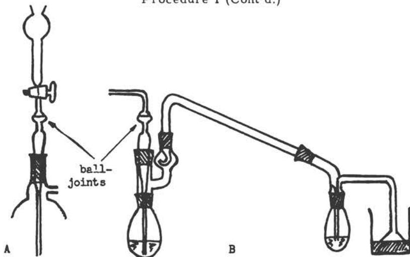
Fig. 8. Apparatus for the distillation of chromium.
