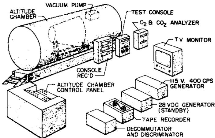
Figure 7. Environmental control system simulator: a device consisting of a mock capsule with a flight-type environmental control system which can be placed within a decompression chamber to simulate the operation of the environmental control system during the Mercury flight.
