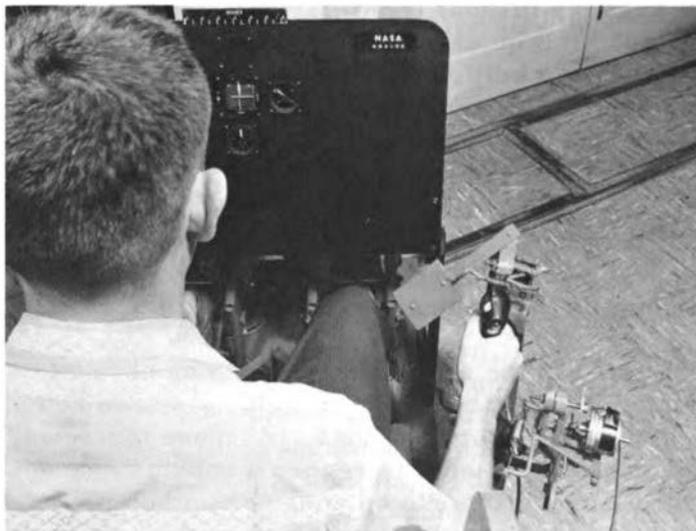
Figure 1. LEAC simulator: a simulator making use of an analog computer on which astronauts were given initial training in attitude control problems.
