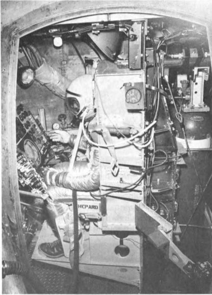
Figure 4. Johnsville centrifuge: centrifuge on which Astronauts were given experience with launch and re-entry acceleration profiles. Note that provisions have been made for use of full-pressure suit and for decompression of the gondola. Astronauts are also provided with simulation of Mercury instrument panel and hand controller.
