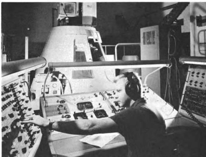
Figure 6. Mercury procedures simulator: a fixed-base trainer which permits practice in management of Mercury systems and attitude control. From instructor's console in foreground, faults can be inserted into any of the Mercury indicators. Astronaut's corrective action is signaled by lights on panel.
