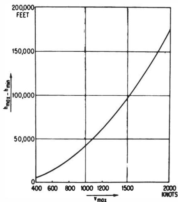
Figure 26. Height of the parabolic arc vs maximal speed, for a minimal speed of 200 knots.
