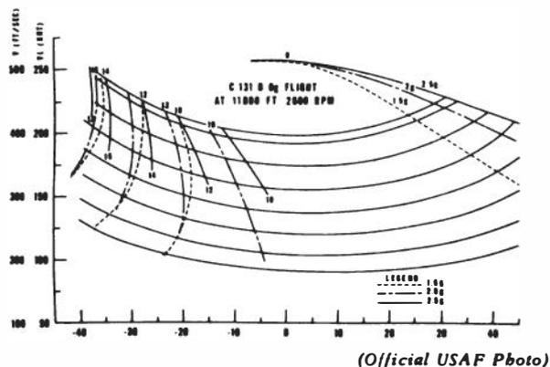
Figure 29. Velocity-Time-Acceleration Nomogram for C-131B Flight Parabolas
