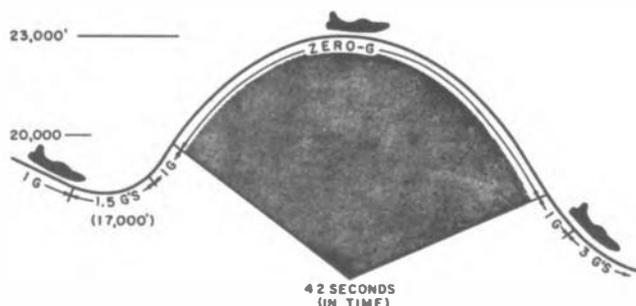
Figure 35. F-94C Zero-G "SAM" Flight Parabola: The maneuver is started at an altitude of about 18,000 feet, reaches about 23,000 feet at the top of the parabola, and yields about 40 seconds of virtual weightlessness.
