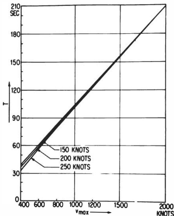
Figure 25. Duration  $T$  of parabolic maneuver as related to maximal and minimal speed.
