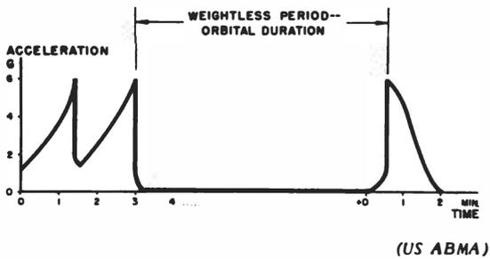
Figure 17. Typical Acceleration Pattern Two-Stage Booster
