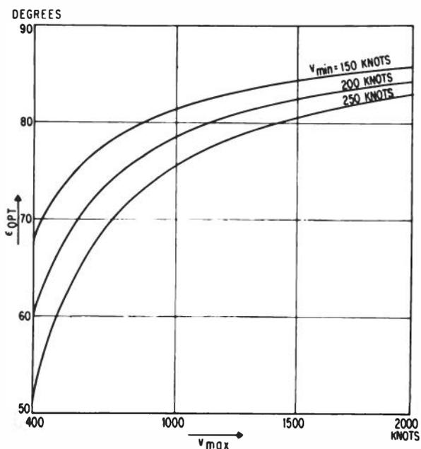
Figure 27. Optimal value of the initial angle of climb as related to maximal and minimal speed.
