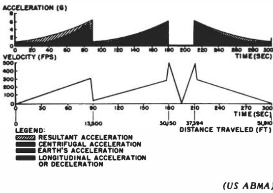
Figure 18. Typical Two-Stage Boosted Capsule
