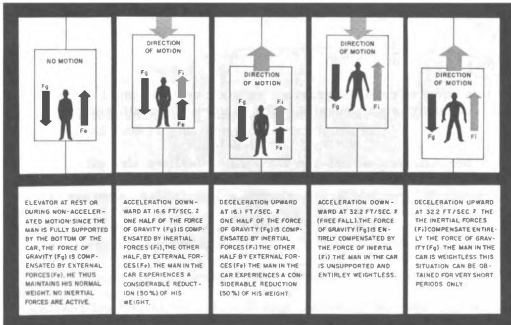
Figure 4a. Sub-gravity and Zero-G in Elevators
