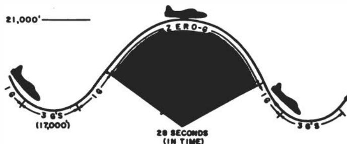
Figure 33. T-33 Zero-G SAM Flight Parabola: The maneuver starts at an altitude of about 18,000 feet, reaches almost 21,000 feet at the top of the parabola, and yields about 28 seconds of virtual weightlessness.
