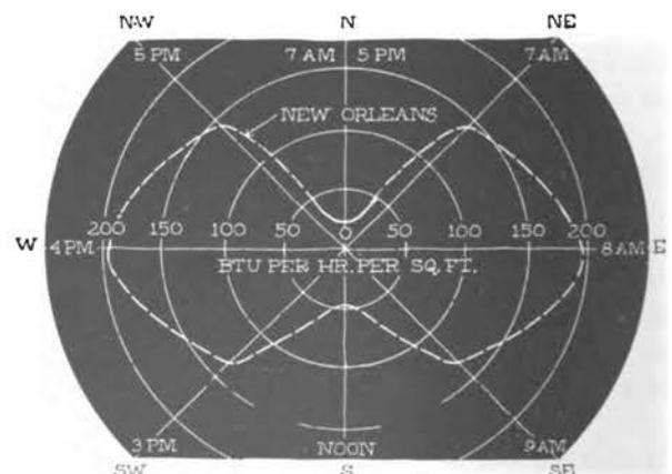
Fig. 3.6—Maximum solar radiation on vertical walls, August 1, New Orleans, La.
