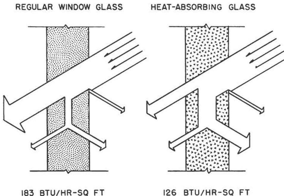
Fig. 1.17—Comparison between regular window glass and heat-absorbing glass.
