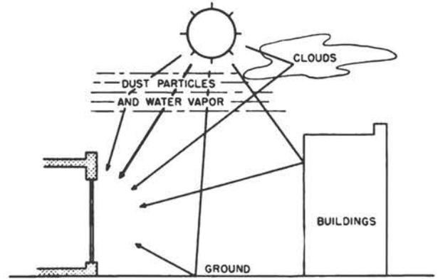
Fig. 1.13—Paths of solar radiation.
