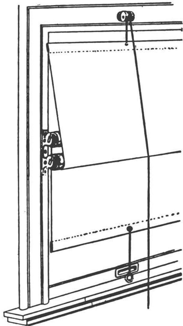
Fig. 3.16—Spring roller shades double hung at center of window.
