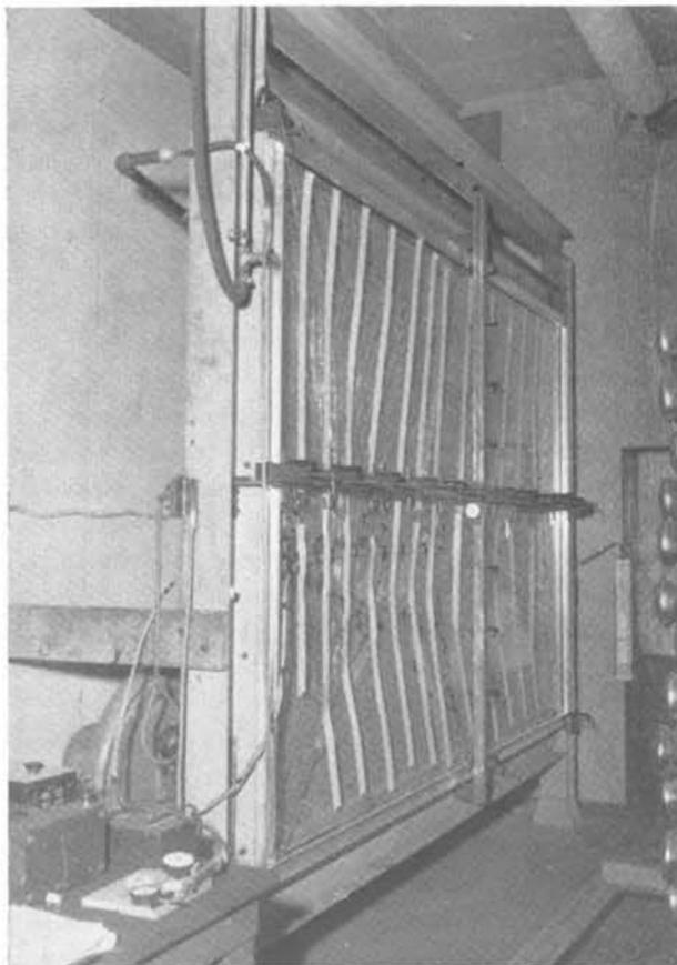
Fig. 2.1—Frame and other equipment used for wind load test of 6'10" x 10' plate.
