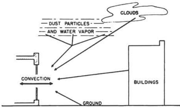
Fig. 1.14—Convection and low-temperature radiation.
