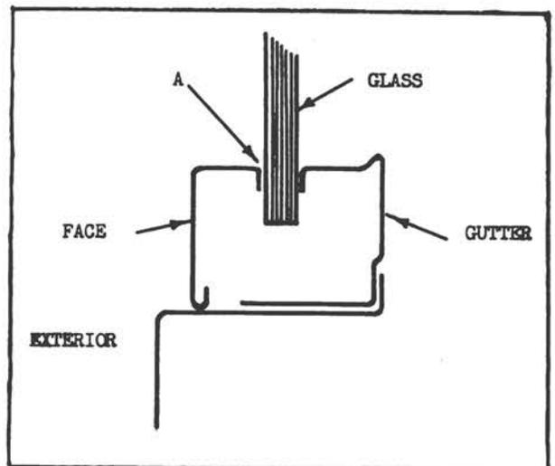
Fig. 2.27—Sash section at sill.
