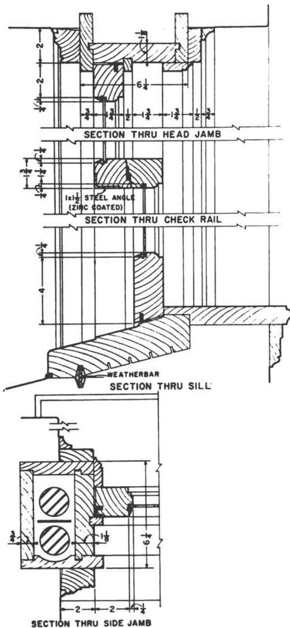
Fig. 2.14—Typical double-hung window and frame for institutional type building.
