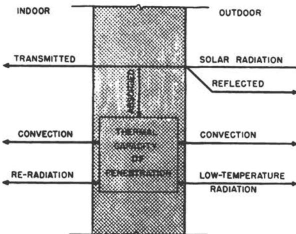
Fig. 1.15—Instantaneous heat balance for any fenestration.
