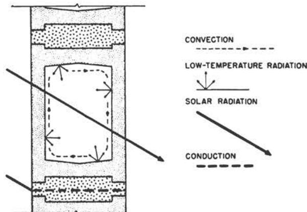
Fig. 1.21—Heat exchanges within a glass block panel.
