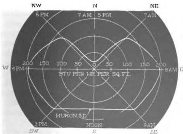
Fig. 3.7—Maximum solar radiation on vertical walls, August 1, Huron, S. D.
