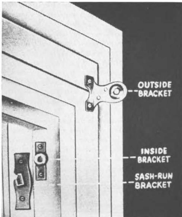
Fig. 3.17—Three types of brackets for installation of spring roller shades.
