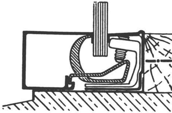
Fig. 4.12—Typical Glazing Molding. (Courtesy of Kawneer Co.)
