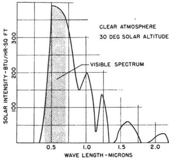
Fig. 1.12—Spectral energy distribution of direct solar radiation at sea level.
