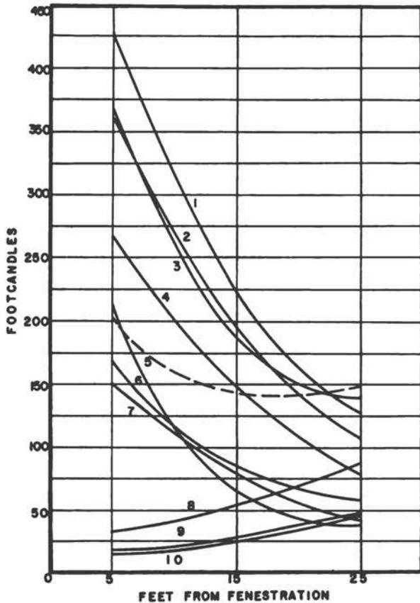
Fig. 1.1—Daylight distribution curves on a thirty-inch work plane.
