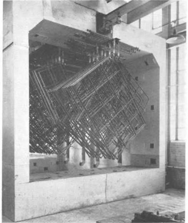
Fig. 2.15—Windows in drying oven after degreasing, pickling, rinsing and fluxing.
