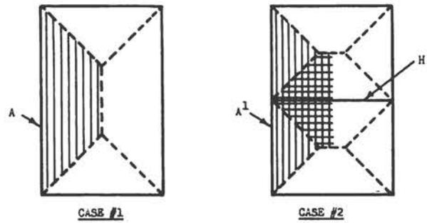
Fig. 2.29—Effect of introduction of a horizontal member.
