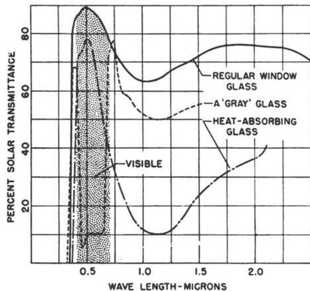
Fig. 1.16—Spectral transmittance of various flat glasses.
