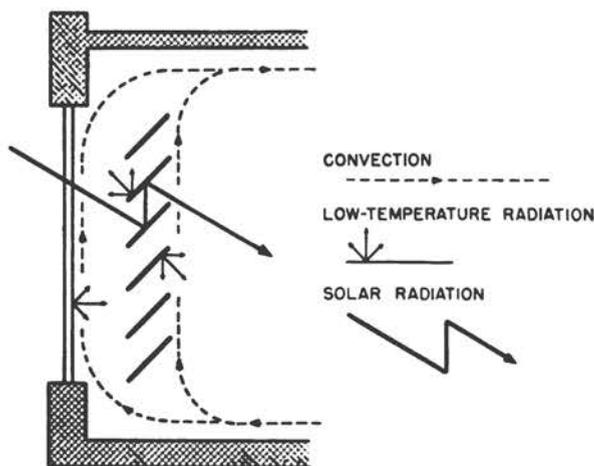
Fig. 1.19—Heat exchanges within a flat glass-venetian blind assembly.
