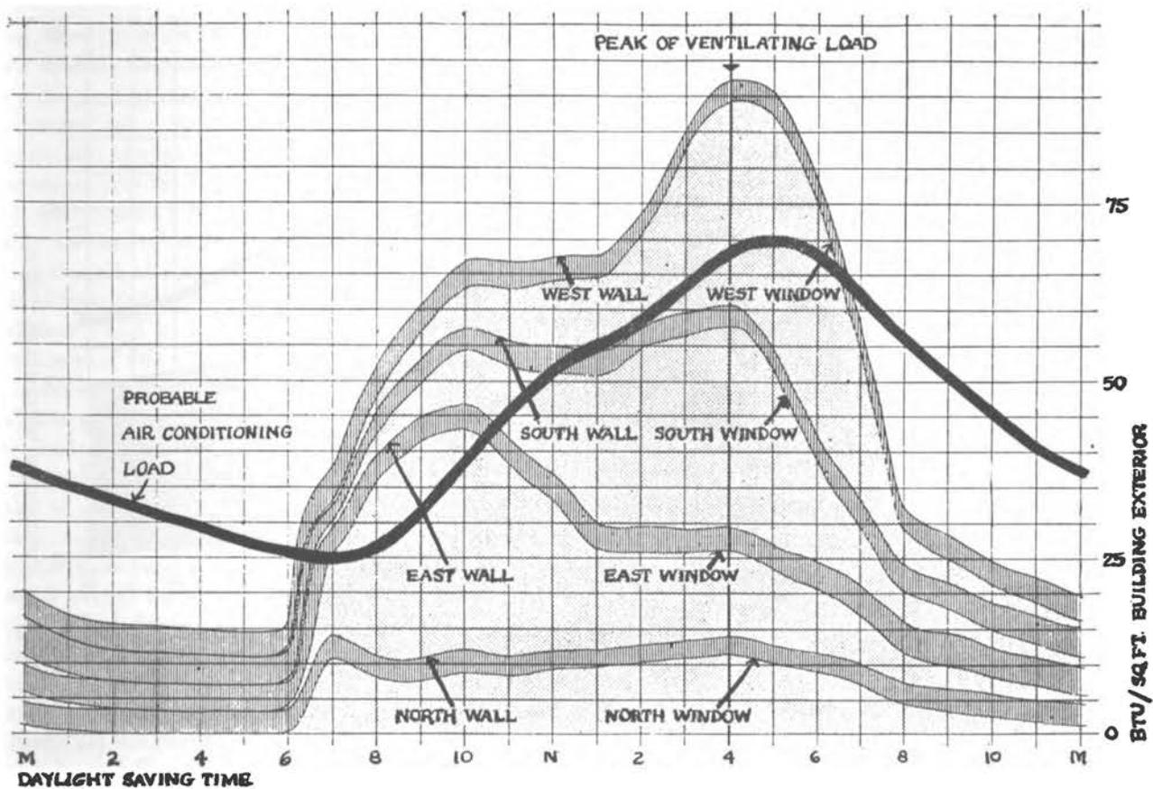
Fig. 3.9—Total instantaneous heat gain due to walls and windows for a square tower with 50% window area, oriented with Manhattan street pattern, August 1.
