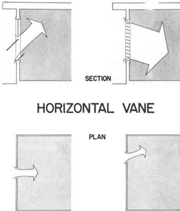
Fig. 1.35—Horizontal vane, section and plan.
