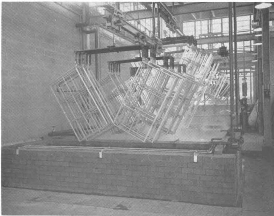
Fig. 2.17—Chemical treatment of windows after galvanizing.
