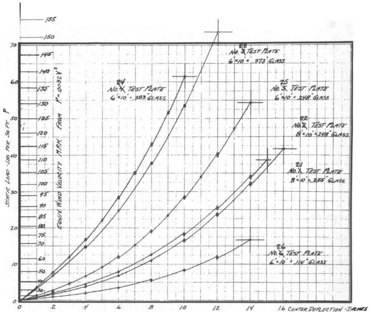
Fig. 2.3—Relation between load and center deflection on large glass plates.
