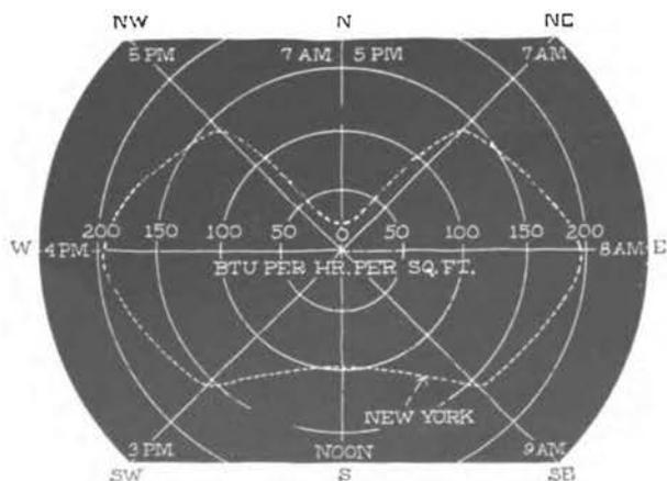
Fig. 3.8—Maximum solar radiation on vertical walls, August 1, New York, N. Y.
