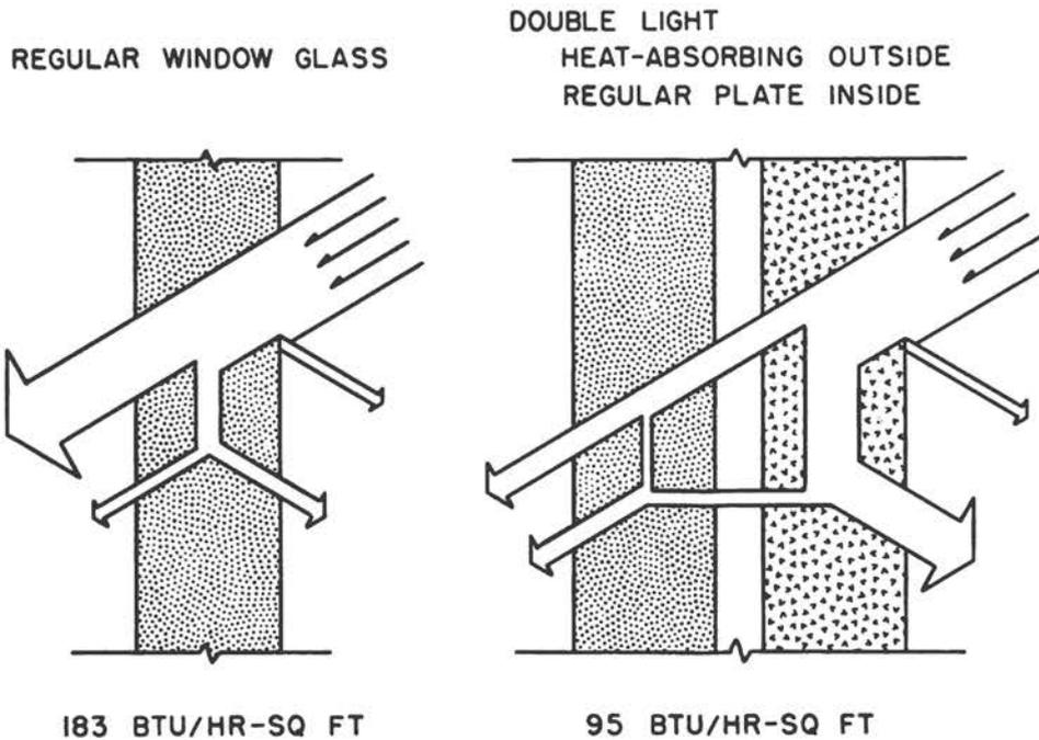
Fig. 1.18—Comparison between regular window glass and a double light.
