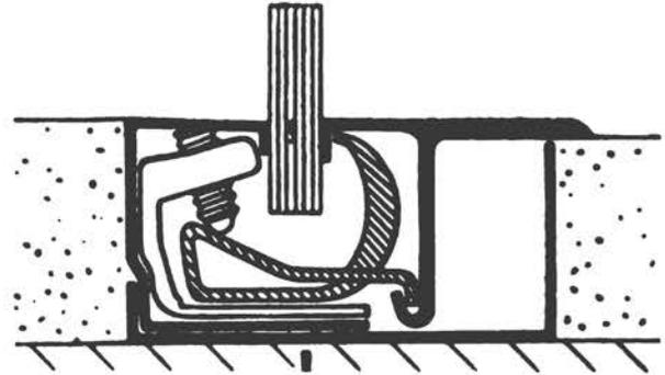
Fig. 4.13—Flush Glazing Molding. (Courtesy of Kawneer Co.)
