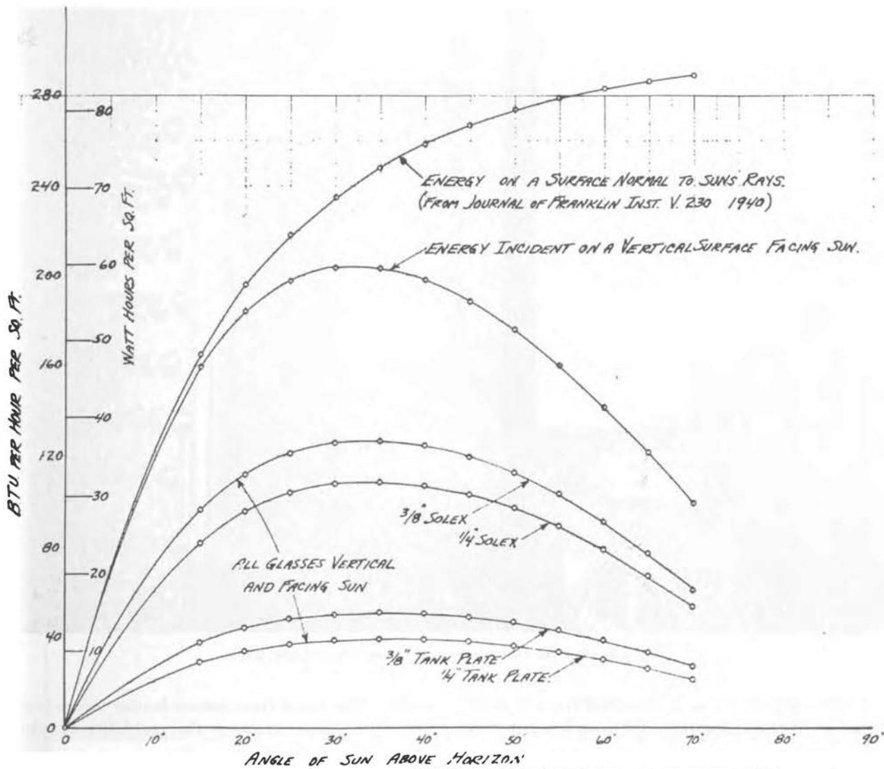
Fig. 2.5—Solar energy available and portion absorbed by various glasses.
