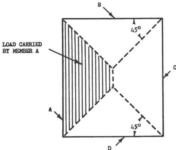
Fig. 2.28—Wind load transmitted to glazing members.
