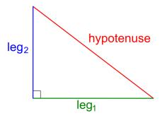
A right triangle is composed of three sides: two legs, which are labeled in the diagram as  $leg_1$  and  $leg_2$ , and a **hypotenuse**, which is the side opposite to the right angle. The hypotenuse is always the longest of the three sides. Typically, we denote the right angle with a small square, as shown above, but this is not required.
