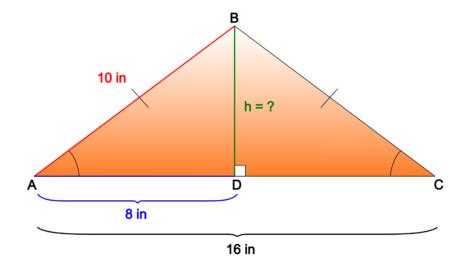
Therefore, we have created two identical right triangles with one leg that is 8 inches long (half of the base) and one hypotenuse that is 10 inches long. Using the Pythagorean Theorem, we can determine the length of the third side, which in this case is the altitude.
