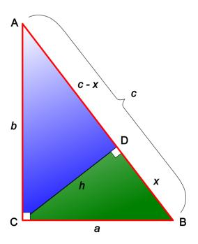
In the diagram above, side *AB* corresponds to side *CB*. Similarly, side *BC* corresponds to side *BD*, and side *CA* corresponds to side *DC*. It is possible to tell which side corresponds to the appropriate side on a similar triangle by using angles; for example, corresponding sides *AB* and *CB* are both opposite a right angle.
